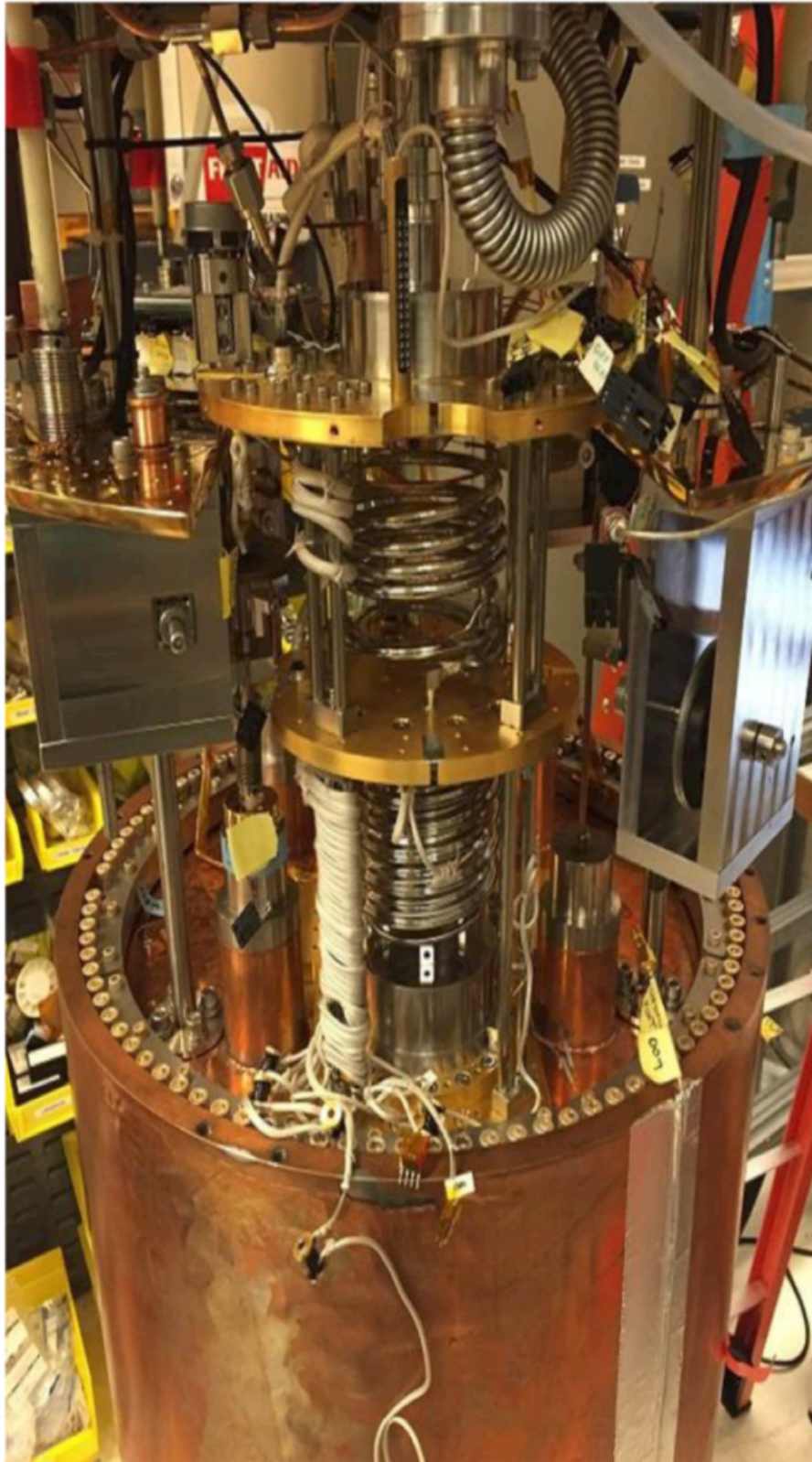
Figure 4.22: Picture of the ADMX DF mixing chambers after installation into the insert. Also in frame are the tuning mechanisms for an antenna (right) and cavity tuning rod (left).
