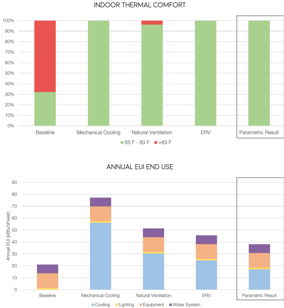
Figure 20. Simulation Result: (a) Indoor Thermal Comfort; (b) Annual EUI End Use
