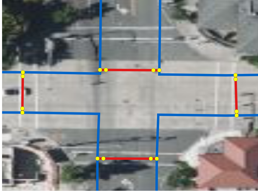
Figure 3.4: Hypothesized graph generated with Pedestrianfer . Yellow dots represent the hypothesized nodes for the curb modes and the nodes on the sidewalk. Blue lines represent the hypothesized sidewalks. Red lines represent the hypothesized crossings. Links are part of the crossings between the curb nodes and the nodes on the sidewalk.
