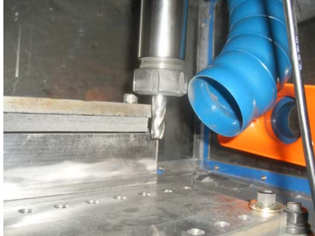
Figure 6.19. Loc-Line Modular Hose relative to cutting tool
