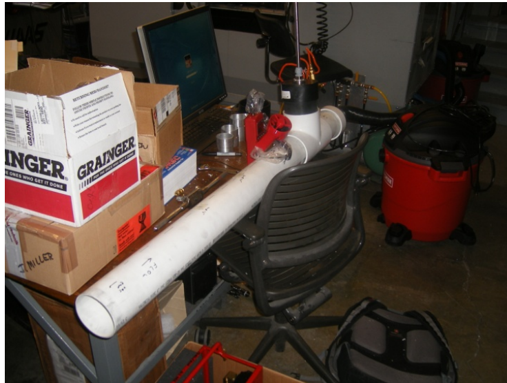
Figure 6.17 Initial isokinetic duct test configuration.
