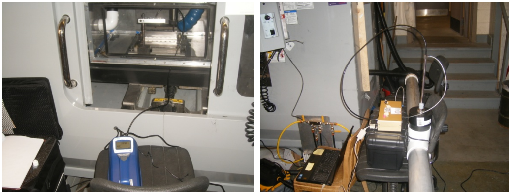
Figure 6.24 GRIMM and PTRAK for first isokinetic test
