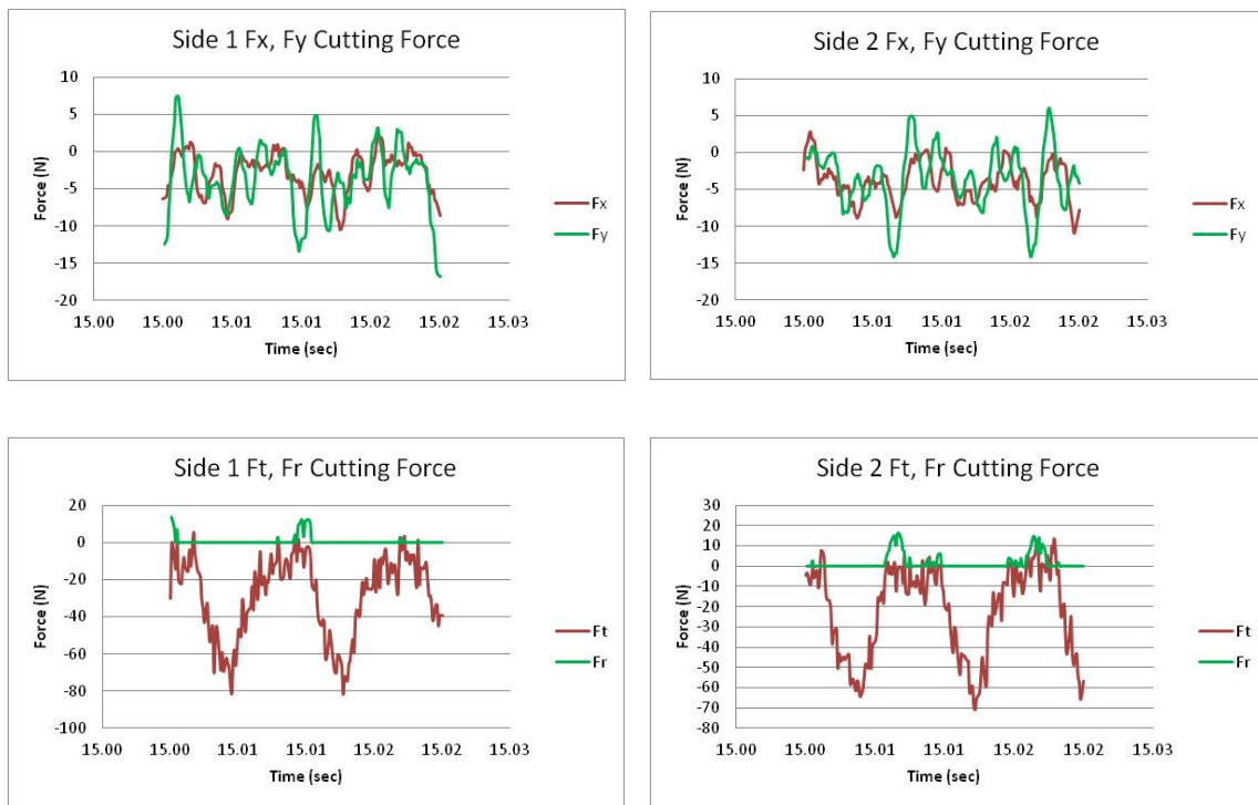
Figure 5.4. Multi-directional laminate cutting forces.
