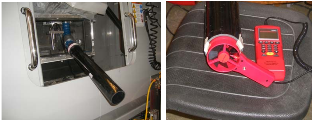
Figure 6.23. Velocity measurement of calibration pipe
