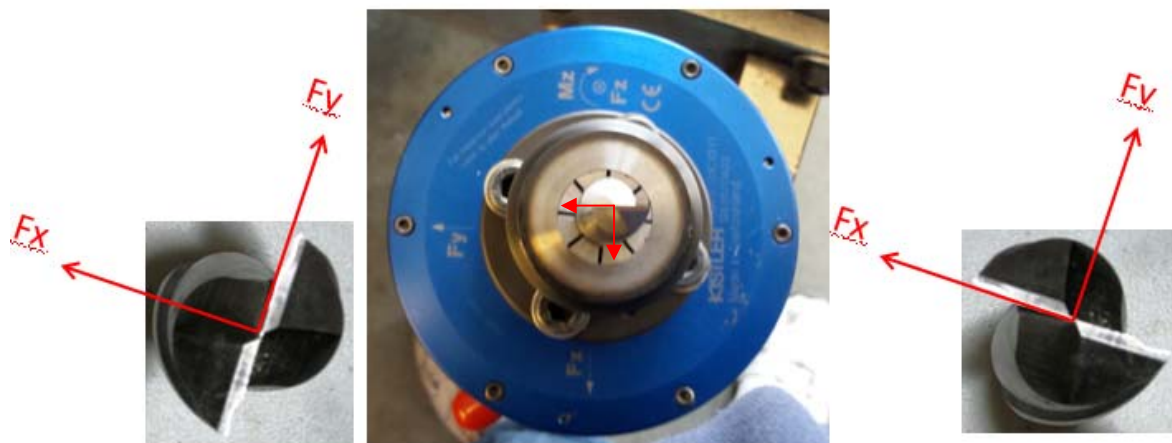
Figure 7.6. Cutting edge relative to dynamometer coordinate system
