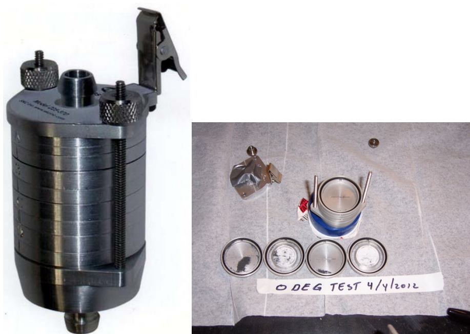
Figure 4.11 Sioutas Cascade Impactor
