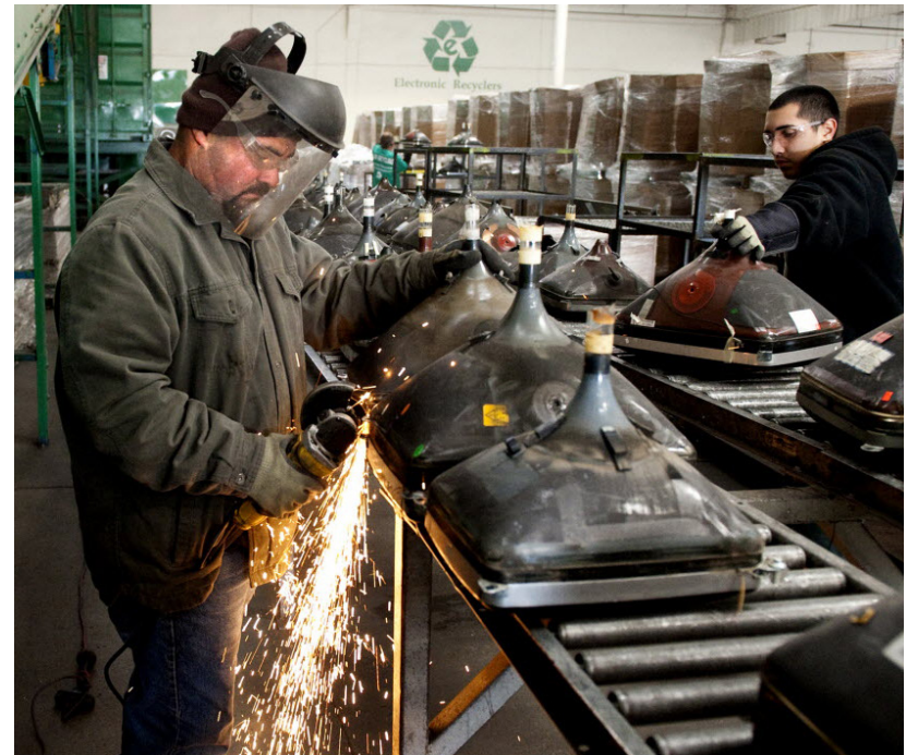
Figure 3.7 Hazardous Work: Manual Disassembly of CRTs
