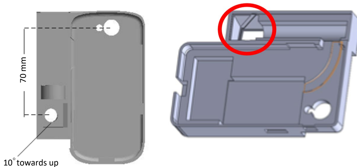
Figure 4.2. (Left) The distance and angle between the camera and laser, and (Right) the DDRS enclosure. The red circle highlights the 2-dimensional angled mirror.
