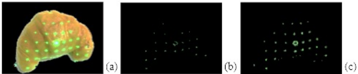
Figure 4.15. (a) Original image (a croissant), (b) croissant image after the luminance mask, (c) second iteration of cosine similarity using dynamic thresholds.
