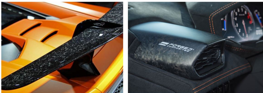
Figure 1.4: Lamborghini forged composite parts, [18,19]
