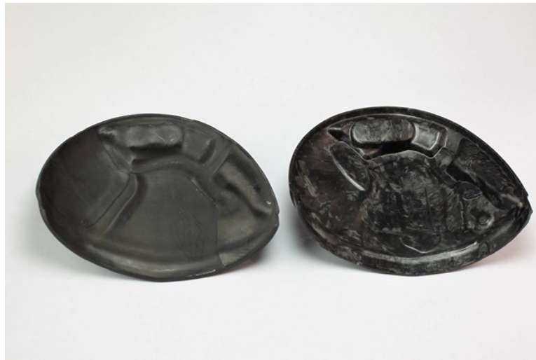
Figure 1.5: Octane driver with the old carbon fiber insides vs Diablo Octane with the Forged Composite technology, [20]
