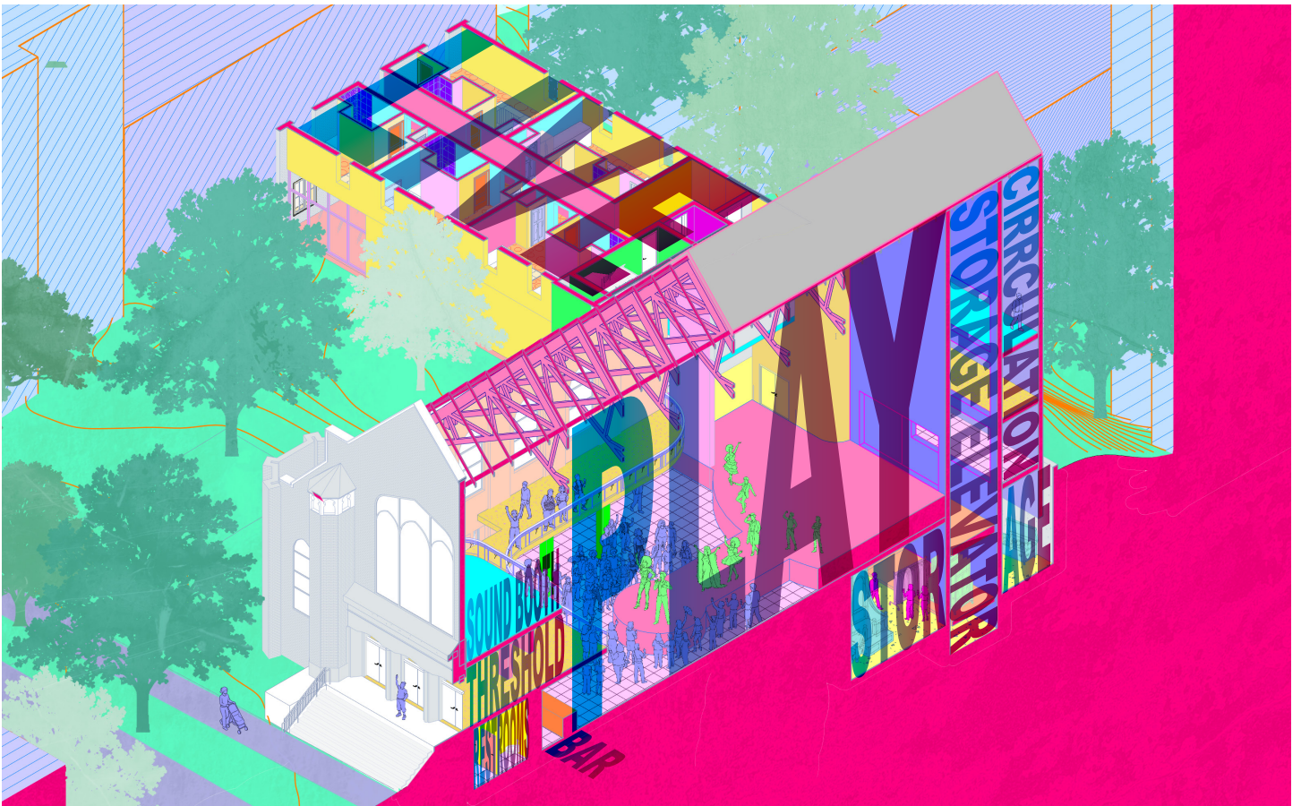
Figure 52: Section axonometric illustrating the spatial organization of the project within the existing church and contemporary addition. The cutaway reveals the primary performance hall, elevated stage, runway, and stage lift, along with backstage support spaces and basement storage located beneath the performance venue.
