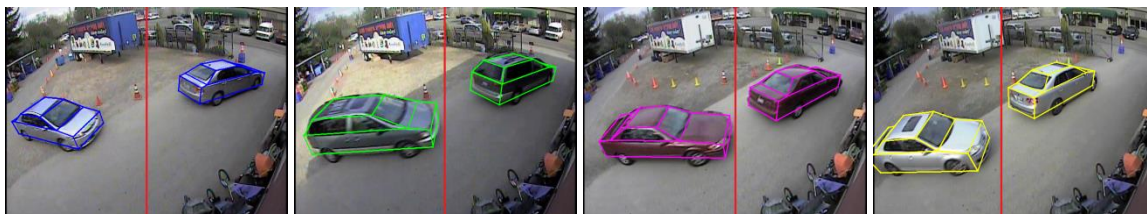
Figure 3.13: The results of 3-D CMK tracking in Dataset 2, where an orientation change of the vehicle happens.
