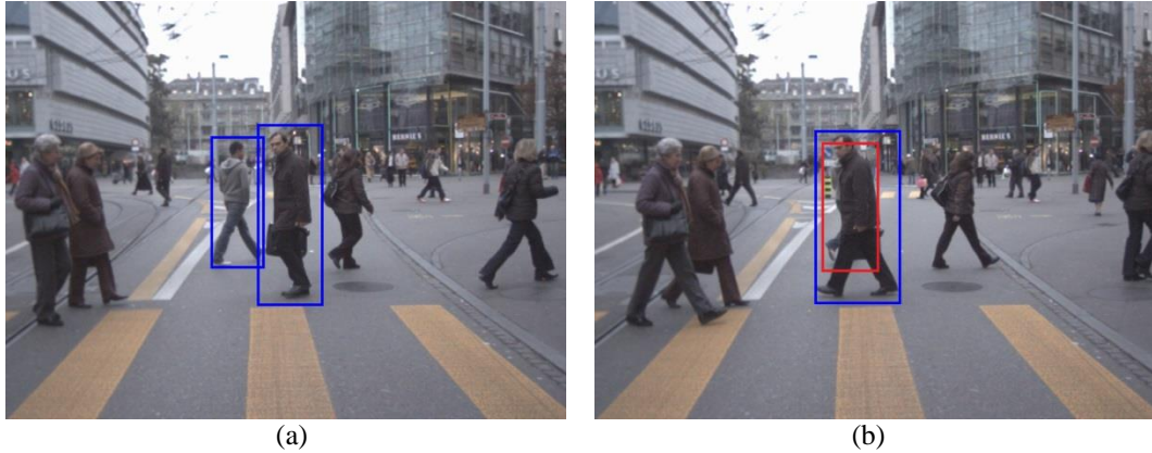
Figure 4.6: An example of the hypothesized association in (a) frame 230 and (b) frame 233; the blue boxes represent the detections, and the red box is the inserted hypothesized association.
