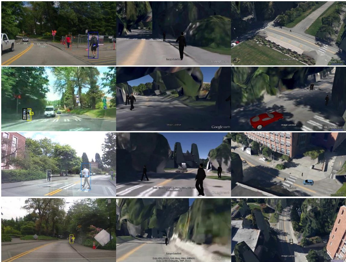
Figure 5.11: 3-D visualization of the scene recorded by four driving recorders. Each row belongs to one driving recorder; the leftmost is the video frames, the middle is the corresponding view of 3-D visualization on Google Earth, and the right is the scene visualized from a different aspect.
