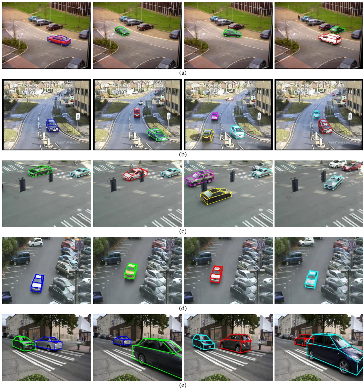
Figure 3.19: A vehicle in PETS 2000 changes its orientation continuously. The results of 3-D CMK tracking in (a) PETS 2000, (b) AVSS 2007, (c) Dataset 4, (d) Dataset 5, and (e) Dataset 6.
