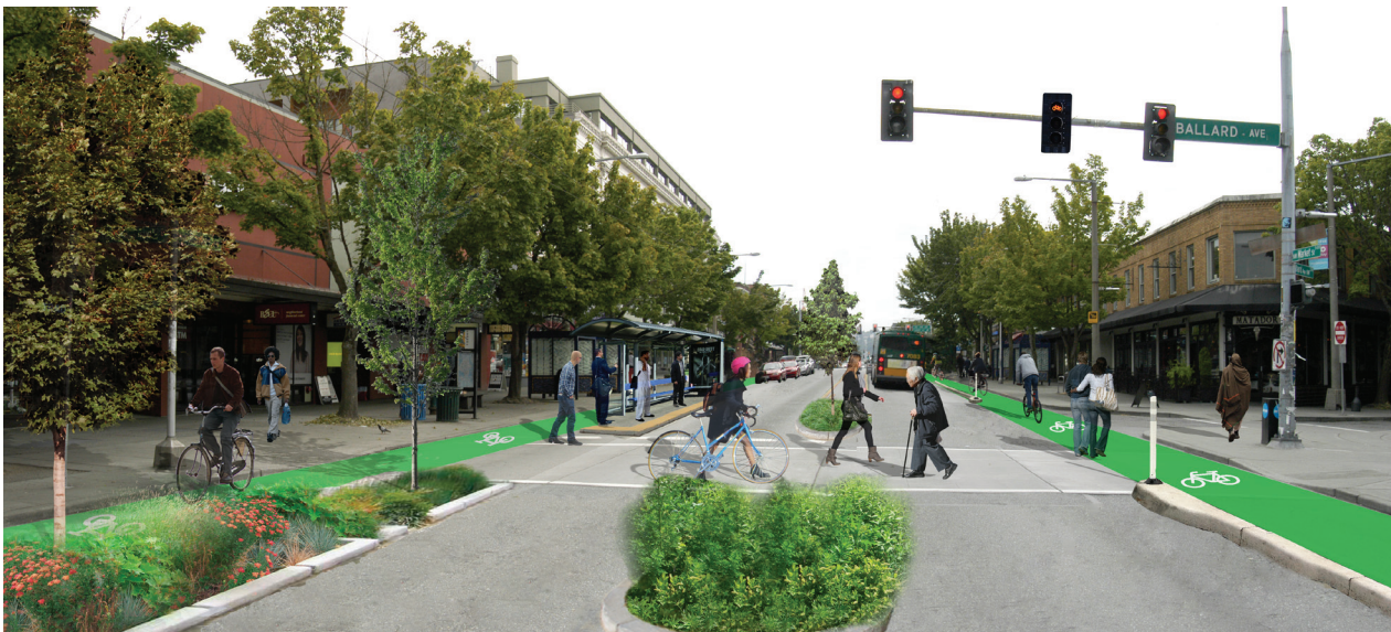
Figure 3A/B. Existing condition of NW Market St (A - top) and author rendering of one-way cycle tracks featuring elements of green stormwater infrastructure (left) and Complete Streets on NW Market St through Ballard (B - bottom)
