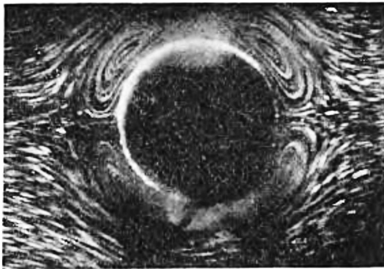
Figure 1. Photograph showing the inner and part of the outer vortex systems near a circular cylinder, radius 0.11 cm. Exposure time 2 sec. Frequency of the sound 200 cps. from Holtsmark, et al. (1954) [50].
