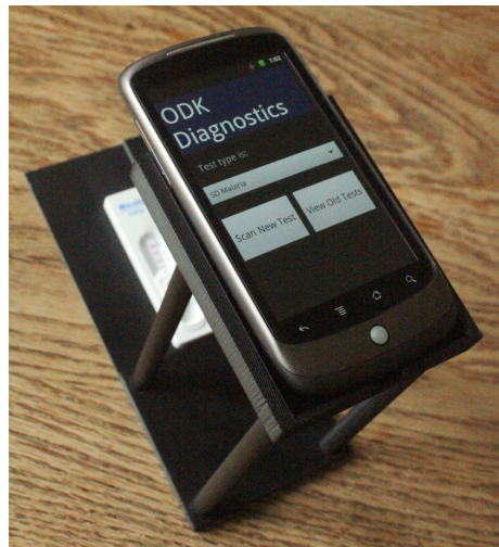
Figure 4.2: Low-cost 3D-printed platform used to capture images of RDTs.
