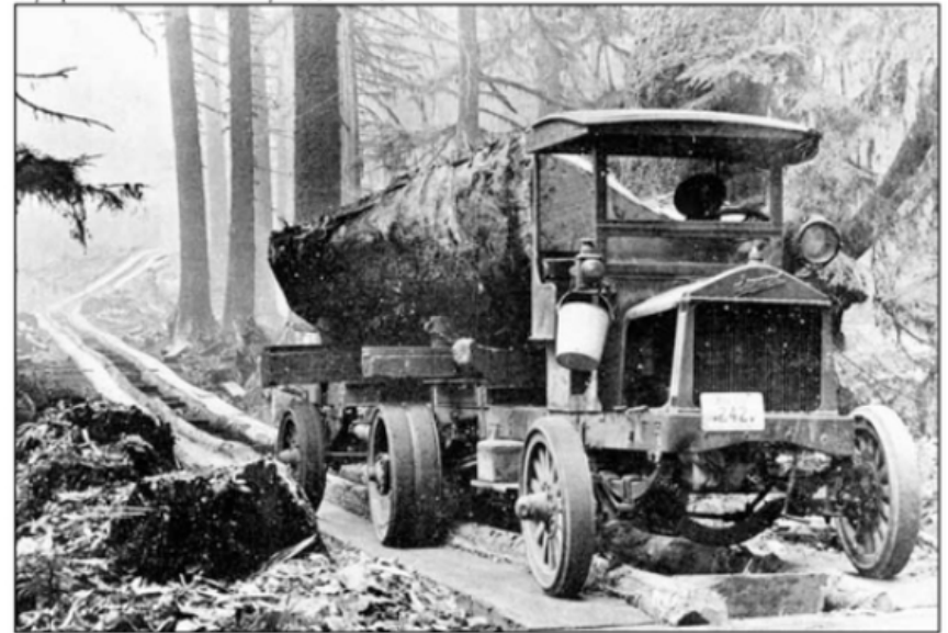
Figure 15: Logging truck using primitive plank roads. [Image Source: Olympic National Forest History Files.]
