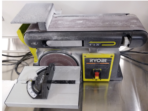
Figure 3.7: Sanding machine used to obtain the chamfered edges
