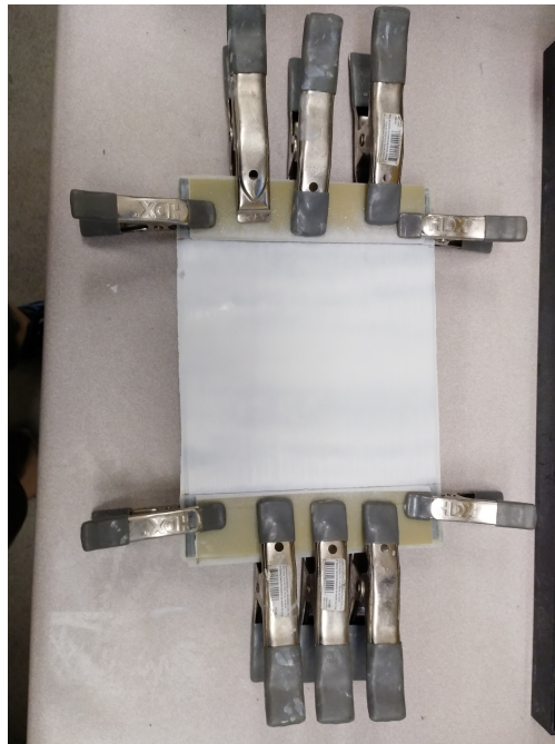
Figure 3.8: The tabs were attached to the gripping section with glue and left for about 16 hours for the glue to cure
