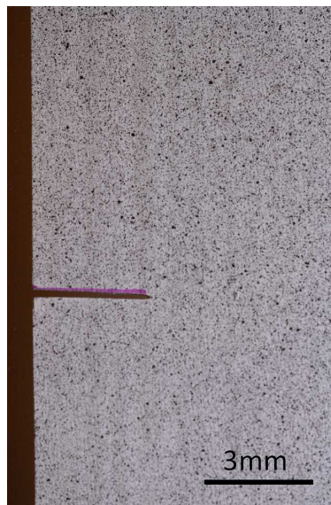
Figure 3.10: Fracture specimen with speckle pattern
