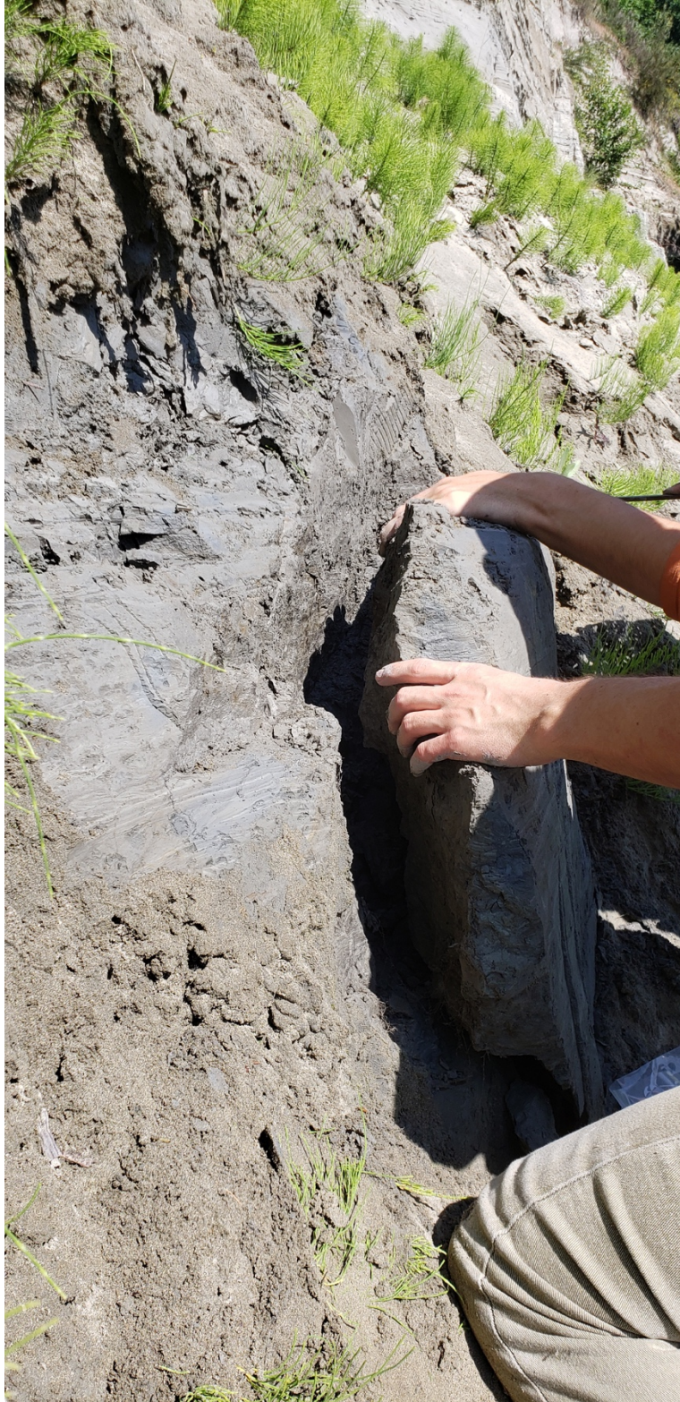
Figure 8. Large block of Lawton Clay extracted from south-southwest exposed bluff at Discovery Park.
