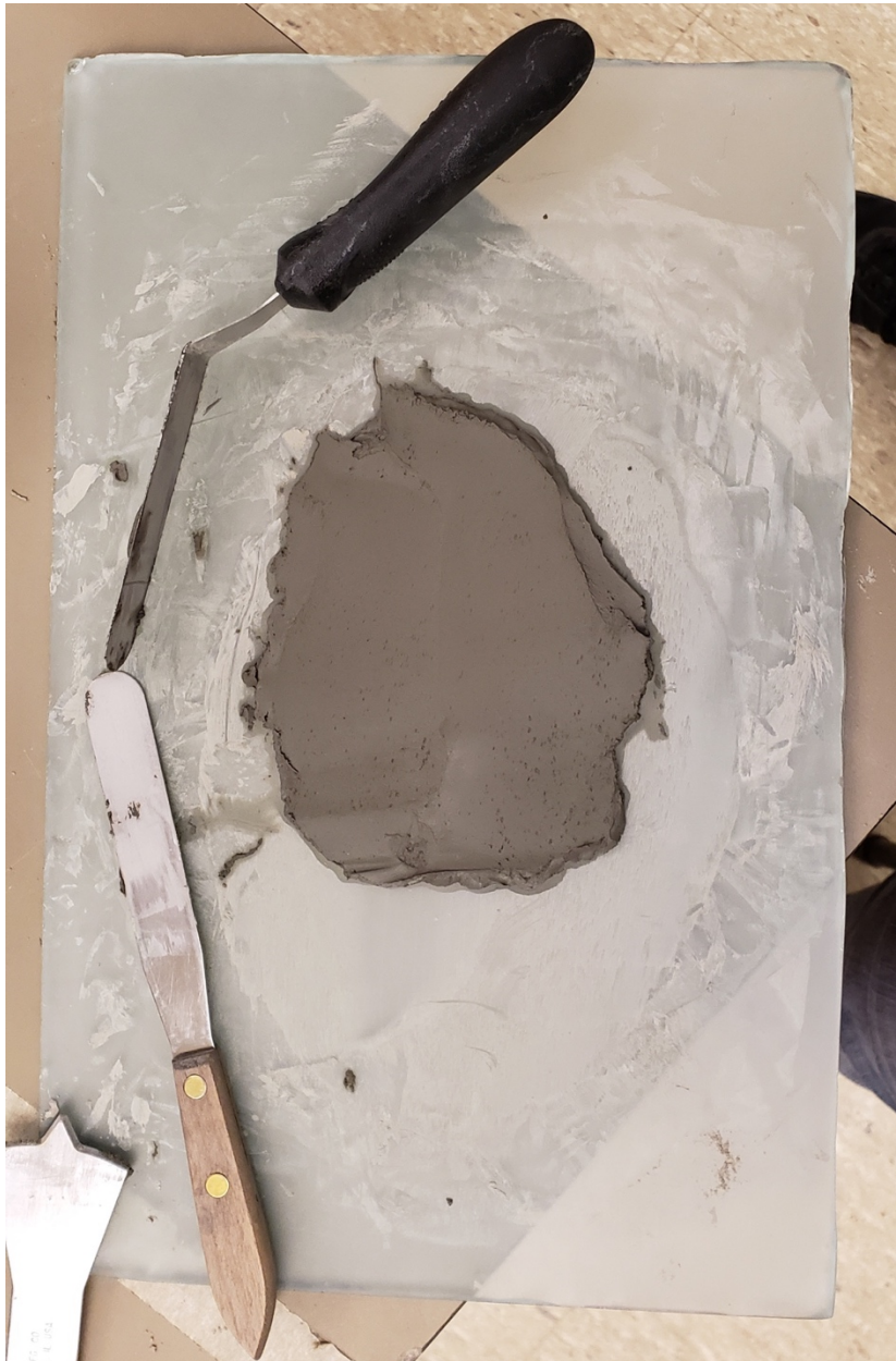
Figure 12. Rehydrated soil pat spread out on frosted glass to lower moisture content.
