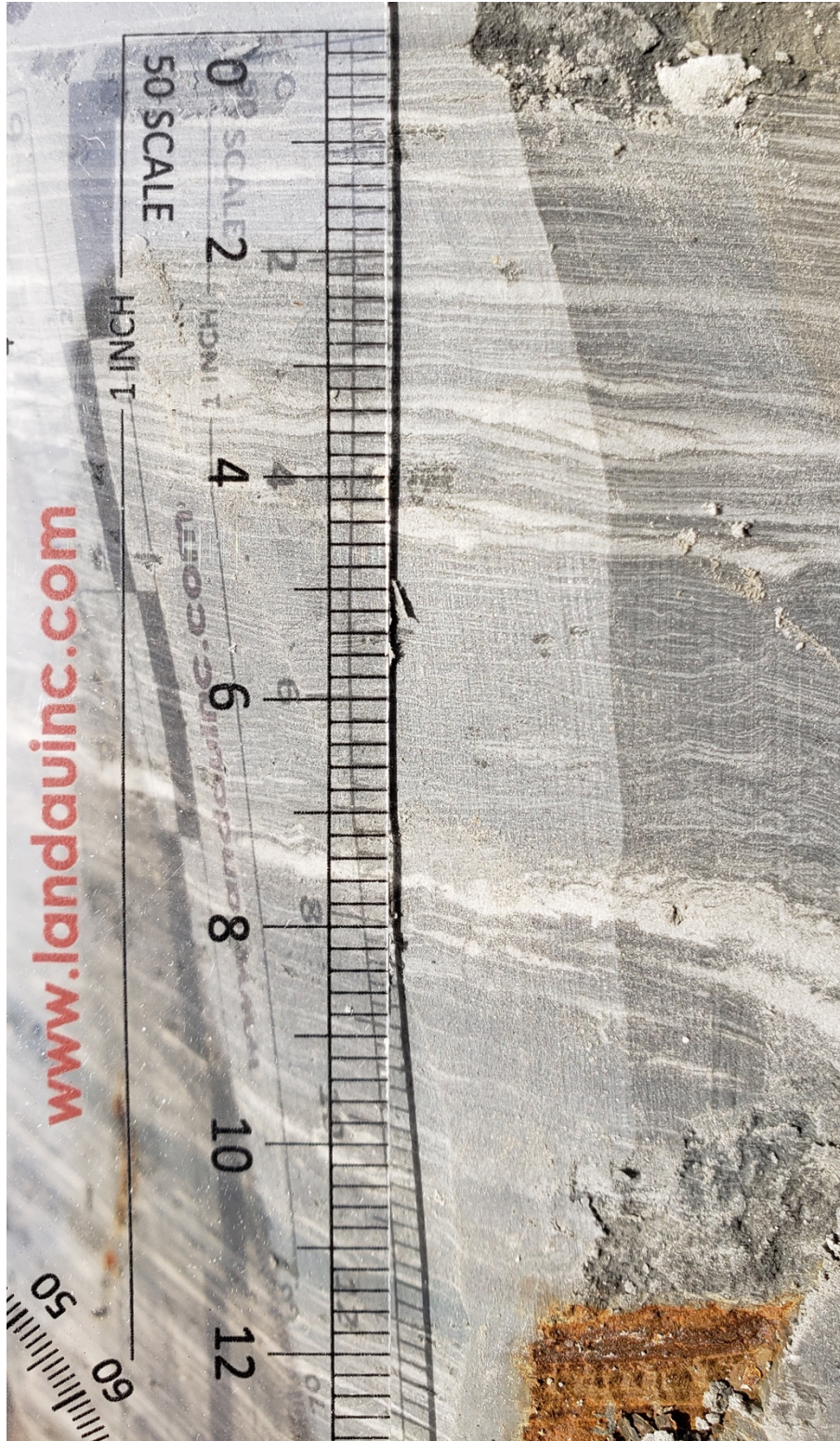
Figure 3. Close up view of the sedimentary structures in the Lawton Clay. Silt appears as thin, light grey layers, while clay layers are thicker and darker grey. There are local ripple marks. Scale is in centimeters.
