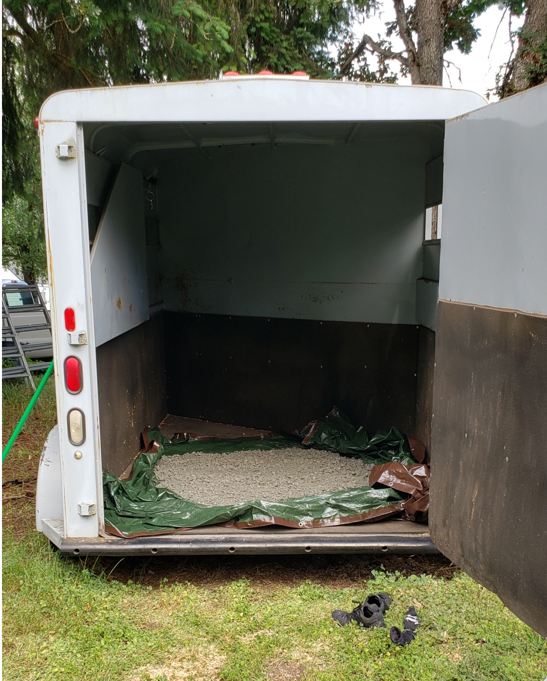
Figure 9. Partially crushed, homogenized sample of Lawton Clay spread out on a tarp in a horse trailer to dry.
