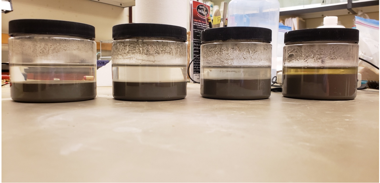
Figure 10. Soil samples rehydrated with sulfuric acid solutions to test buffer capacity. The pH of the samples are 2.52, 1.91, 0.92, and 0.0 from left to right. Each sample has 200 mL of solution and 120 g of soil. Notice the decreased consolidation at lower pH values.
