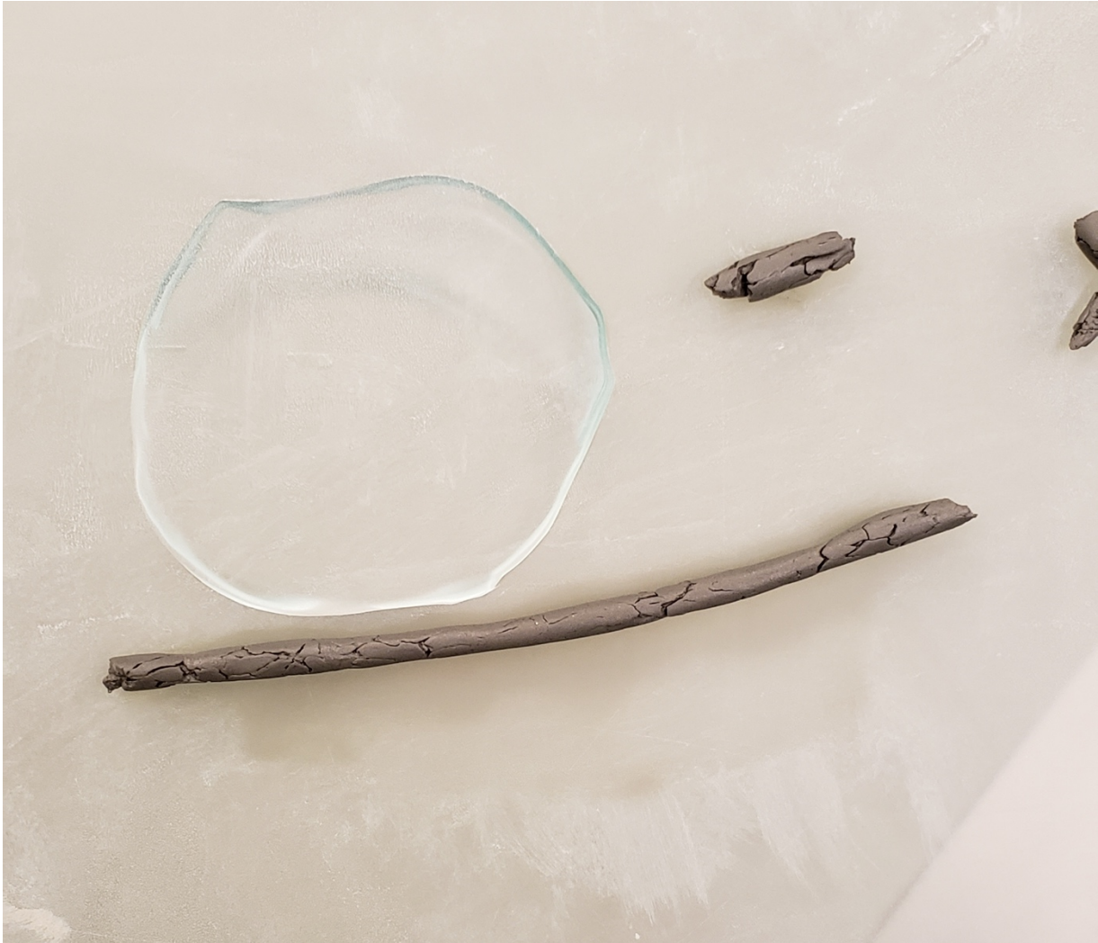
Figure 13. Thread of soil breaking apart at a diameter of 3.2 mm (~1/8 in.). This thread is at the plastic limit.
