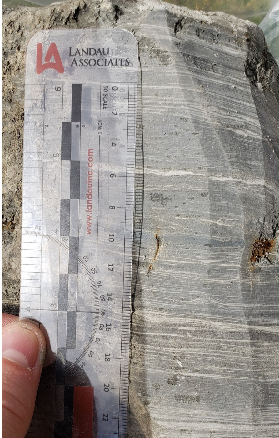
Figure 2. Block sample of Lawton Clay consisting of laminated clay and silt. Silt appears as thin, light grey layers, while clay layers are thicker and darker grey. There are local ripple marks. Scale is in centimeters.
