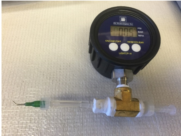
Figure 32: SSI Technologies gauge with precision 0.01 psi to measure air pressure
