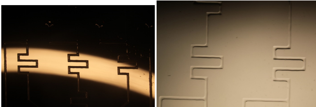
Figure 47: AZ-50XT mold on wafer (left) of oscillator with corresponding embossed pattern on PMMA (right)
