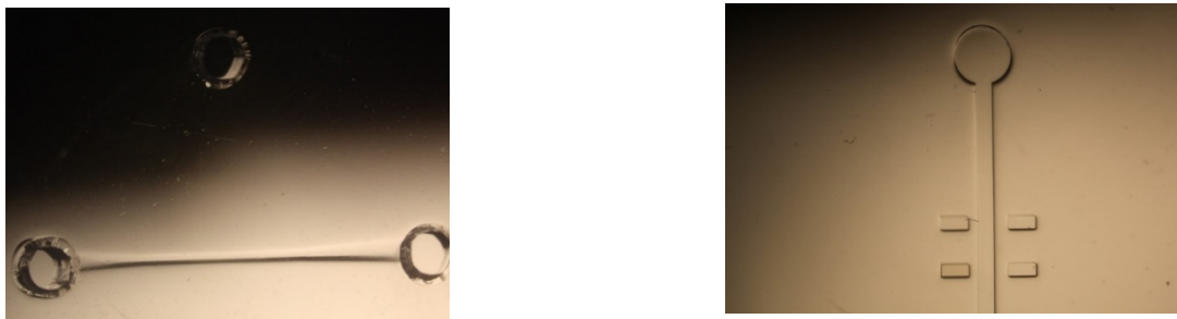
Figure 34: Embossed (left) (110°C, 250lbs) flow channel of dimension 300um(W)x35um(H) with holes drilled for inlets; Embossed (right) (113°C, 270lbs) of dimension 500um(W)x47um(H)
