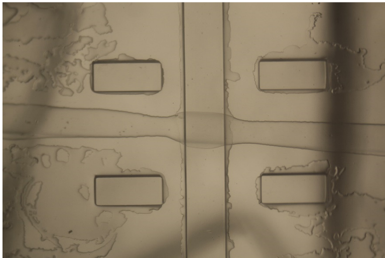
Figure 36: Bonded Quake valve with membrane of thickness 50um
