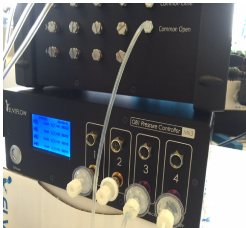
Figure 66: Elveflow pressure controller (left) for applying constant vacuum supply and (right) frequency of oscillations varying with magnitude of vacuum applied
