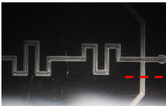
Figure 57: Milled 300um channel oscillator with capacitor in feedback circuit (top) along with height profile of resistor and outer channel (bottom).
