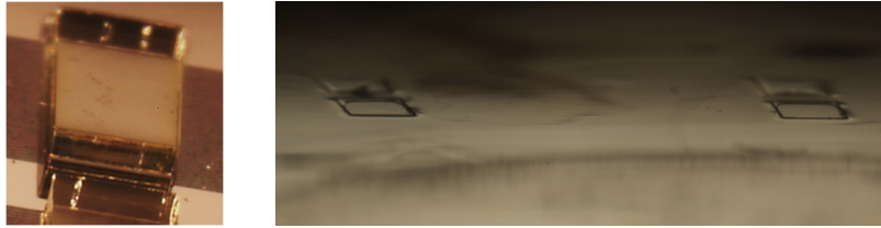
Figure 12: Cubic structures on SU-8 300um tall (left) and corresponding imprint on PMMA (right)
