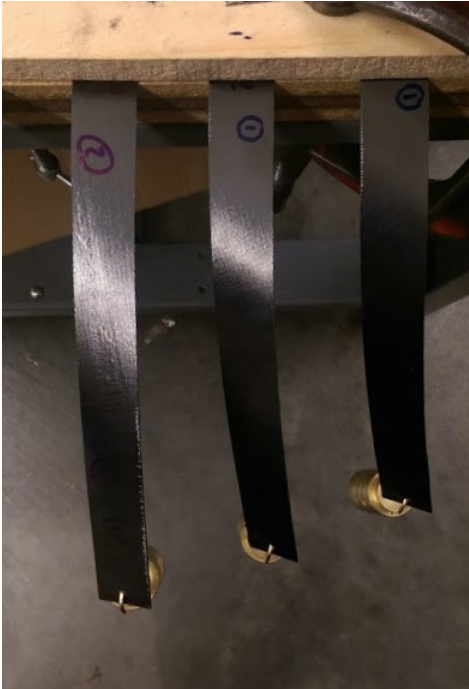
Figure 2.4: Deflection of varied fiber angle ( 10^\circ , 20^\circ , 30^\circ ) beams under identical loading
