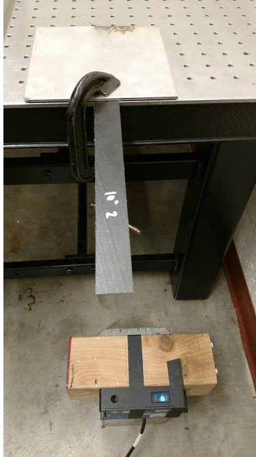
Figure 2.5: Experimental setup for free vibration
