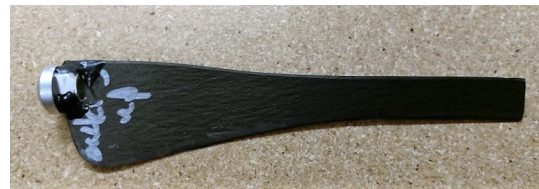
(b) Spar cut by Dremel from cured laminates
