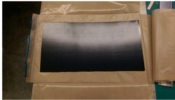
(a) Finished cured laminate from hot press
