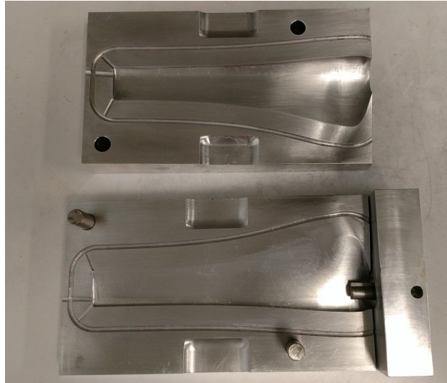
Figure 5.3: Machined aluminum mold of flume-scale blade geometry
