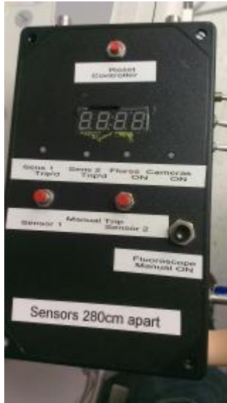
Figure 3.1. The Arduino control box housing the microcontroller with controls and indicators on the top to manipulate the system.
