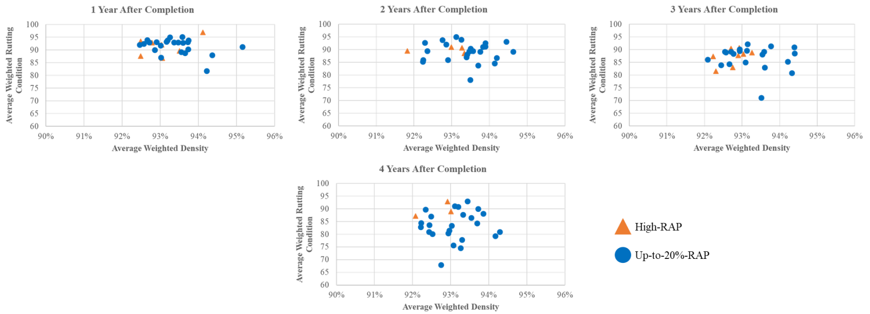
Figure 58. Average Weighted Pavement Rutting Condition Versus Average Weighted Density by Number of Years After Completion for High-RAP and Up-to-20%-RAP WSDOT Asphalt Pavement Mixtures, 2013 to 2016
