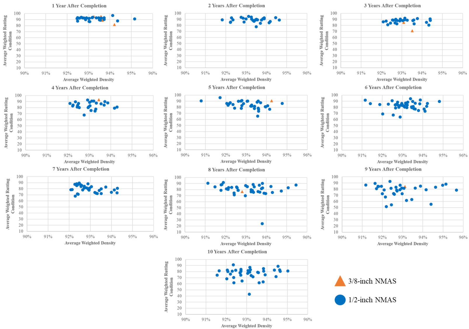
Figure 43. Average Weighted Rutting Condition Versus Average Weighted Density by Number of Years After Contract Completion and NMA for WSDOT Asphalt Pavement Mixtures, 2007 to 2016
