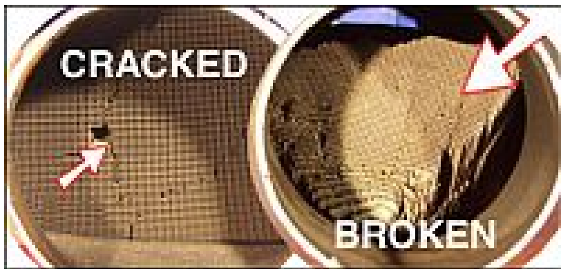
Figure 1.5: An example of cracked catalytic converter and broken catalytic converter. Image courtesy of Davis Recycling Inc [8].
