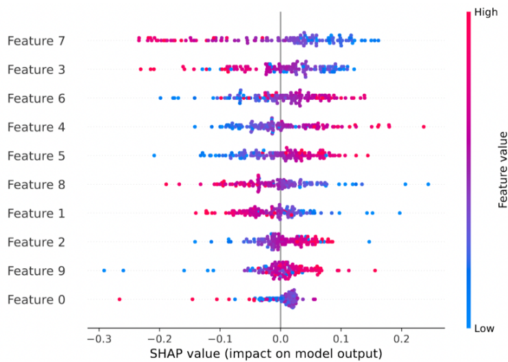
Figure 3.8 SHAP Summary Plot of All Features. This figure illustrates the impact of each feature on the model’s predictions, with features ranked by importance from top to bottom.
