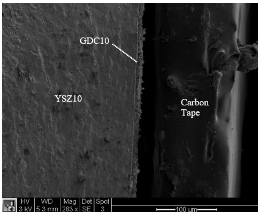
Figure 3.4. SEM of painted porous GDC10 electrode on YSZ10 pellet.
