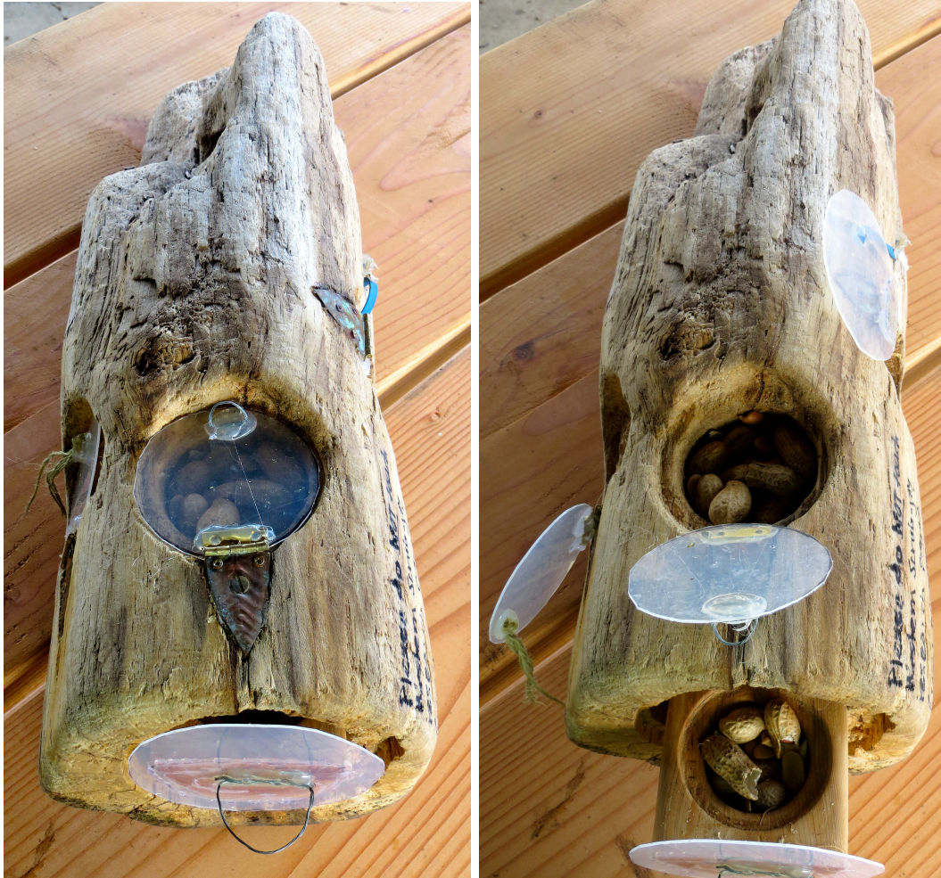
Figure 1: We created our puzzle box from a log by carving out 4 compartments and covering them with clear doors that open in different ways. The top door opens up like a hatch. The left door opens out like a car door. The front door pulls out like a drawer, and the door on the right side of the log has a hinge at the top and so pushes in (in the right photo it is pulled up for the open, habituation phase).
