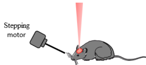
Figure 6. Schematic illustration of whisker stimulation with a stepping motor.
