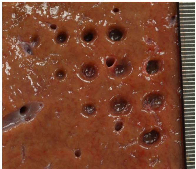
FIGURE 3.10: Photograph showing the typical erosion pattern on the liver surface. From left to right on each line (the final line is split into 2 lines), exposures were completed in the order A (10 pulses), B (30 pulses), C (60 pulses), and D (120 pulses). The first exposure A in the upper left corner occurred on a vessel, so that exposure was excluded from the erosion analysis.
