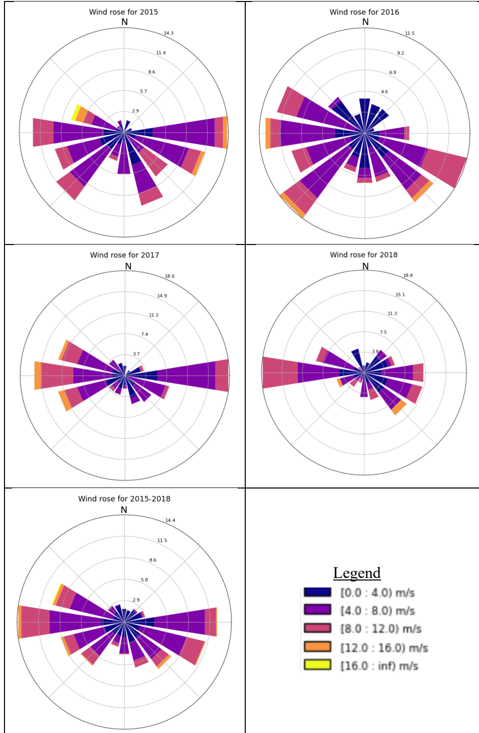
Suppl. Fig 2: Wind rose, based on daily wind speed and wind direction, for each year (2015 - 2018) from 1 October until that year's survey date. The last windrose, in the bottom left, is from 1 October to 31 March for 2015 to 2018. The value on the different rings of the windrose is the percent of time the wind blew from that direction during the time-period.
