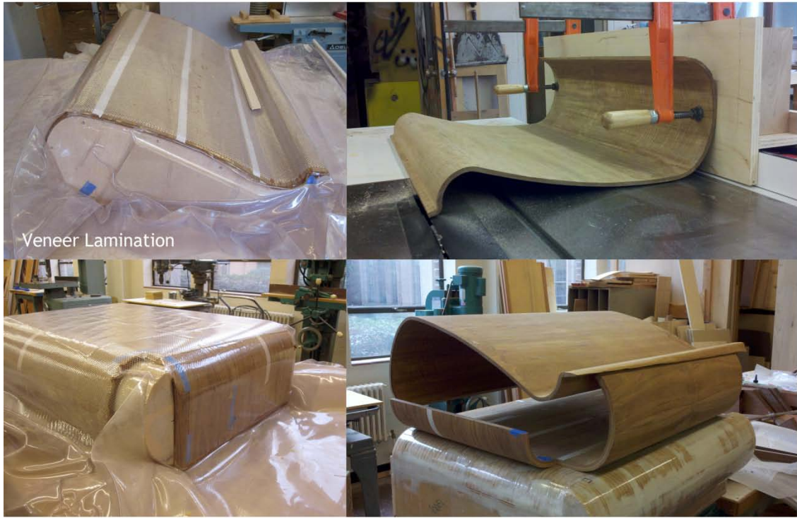
Using cut-patterns of teak and mahogany veneer with a single-sided mold/vacuum bag process.
