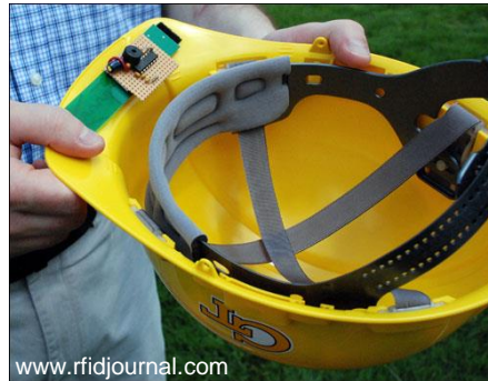
Figure 4: RFID Tag Attached to a Hard Hat
