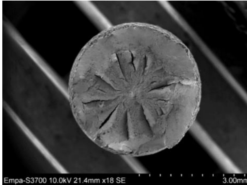
Figure 6.6: Fracture surface of a wire from the SE stay showing fatigue damage, from [Rosati et al. (2018)]
