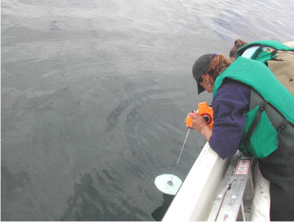
Figure 7. Taking a vertical secchi disc depth to measure water visibility.
