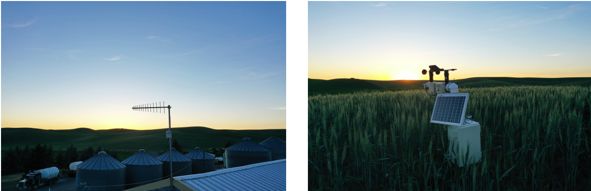
Figure 2.10: Nelson Farm Deployment. A TV whitespace base station and FarmBeats sensor box deployed on Nelson Farm.
