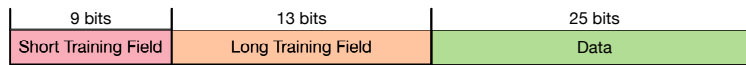
Figure 4.4: Packet Structure for Glaze Embedding. The Glaze system uses a short and long training field, followed by data, to overlay packets on top of existing signals.
