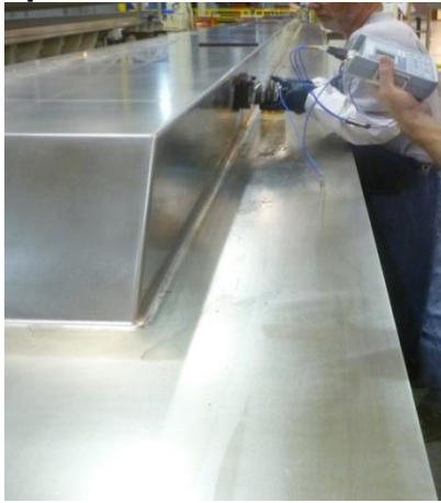
Figure 4: An actual LM Spar being sanded by a subject during normal work-day operations.
