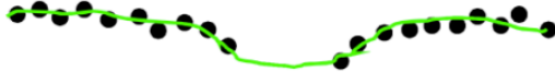
Figure 20. Example of a cloud of points at a concavity with low point density, and the corresponding surface generation
