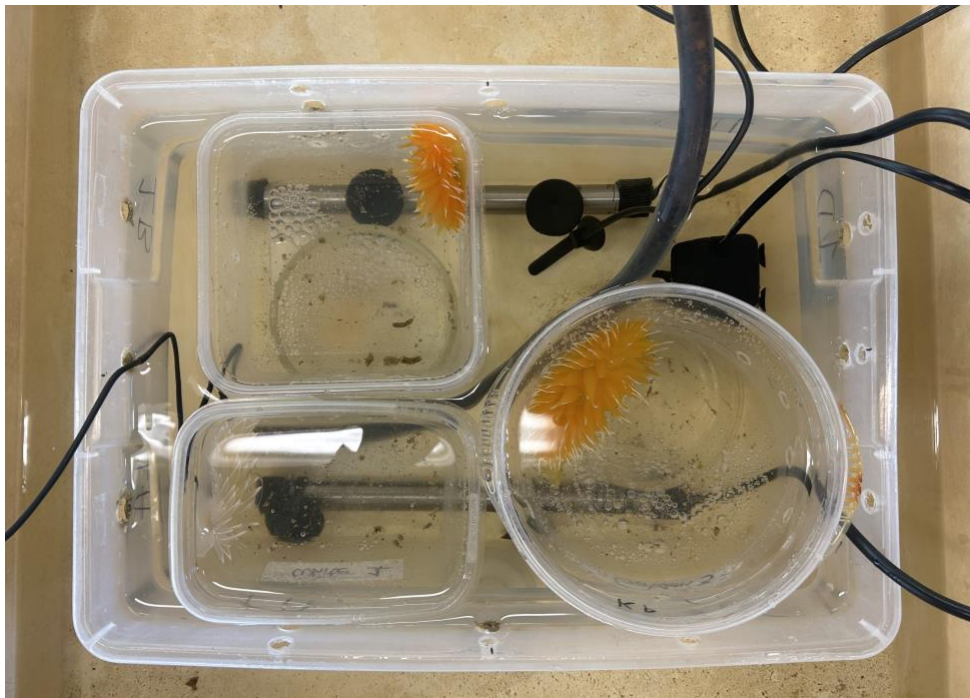
Figure 1. Feeding trial sea table layout. A larger container was placed inside the sea table with two heaters at the bottom and a water pump attached to the side. Where nudibranchs were placed in individual mesh-sided containers with a constant flow of fresh seawater.
