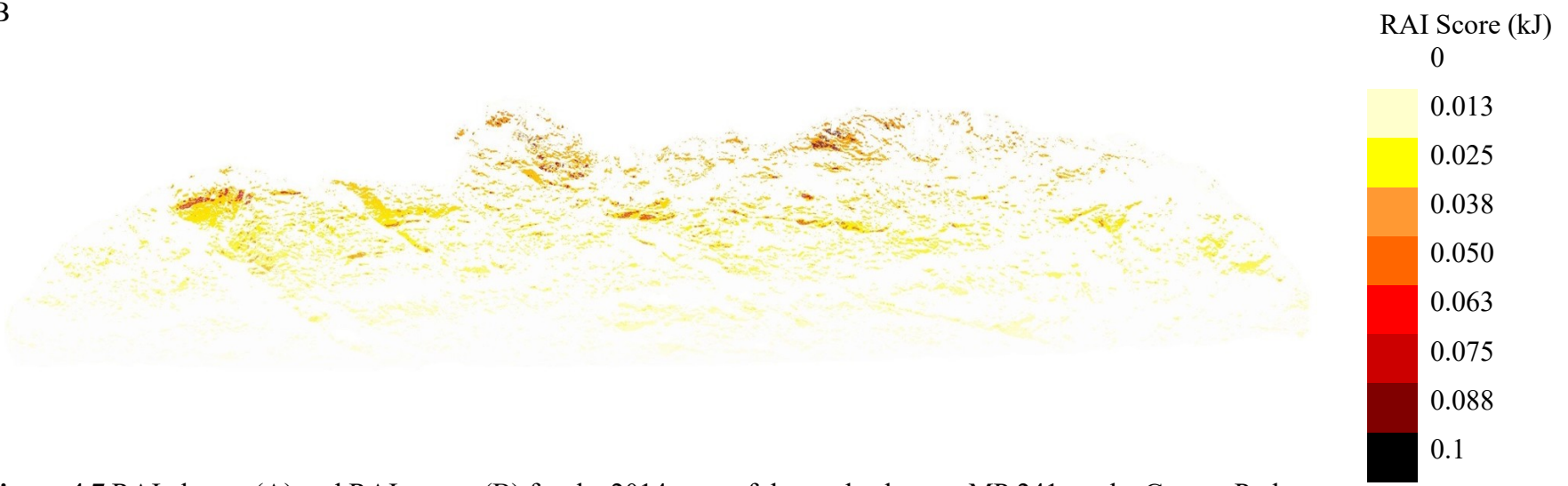
Figure 4.7 RAI classes (A) and RAI scores (B) for the 2014 scan of the study slope at MP 241 on the George Parks Highway near Glitter Gulch, Alaska.
