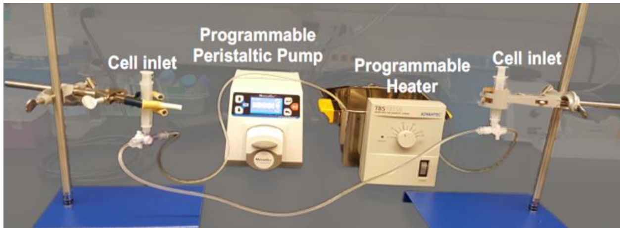
Figure 3.2. Arrangement of in vitro CPB circuit. The circuit consists of PVC tubing, cell inlets, a peristaltic pump, and a programmable heater. Cells are loaded in the inlet, propelled by the peristaltic pump. The heater is used to maintain the temperature of the cell suspension.
