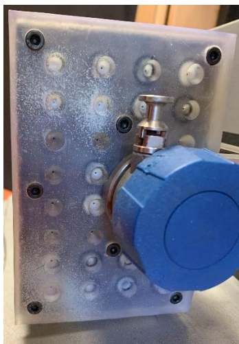
Figure 9. The contents inside the reaction vials sprayed out of the injection sites after ball mill processing.
