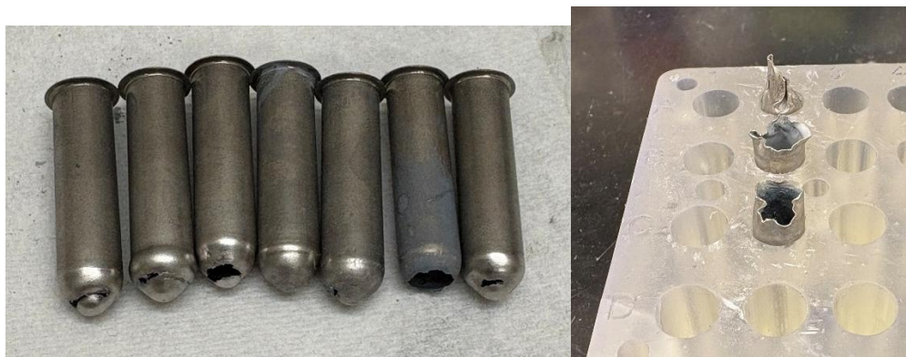
Figure 16. Aluminum vials with perforations after ball mill processing (left) and lodged inside a reaction vial holder (right).
