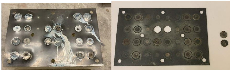
Figure 15. The original reaction vials caused leakage and perforations in the EPDM elastomer.
