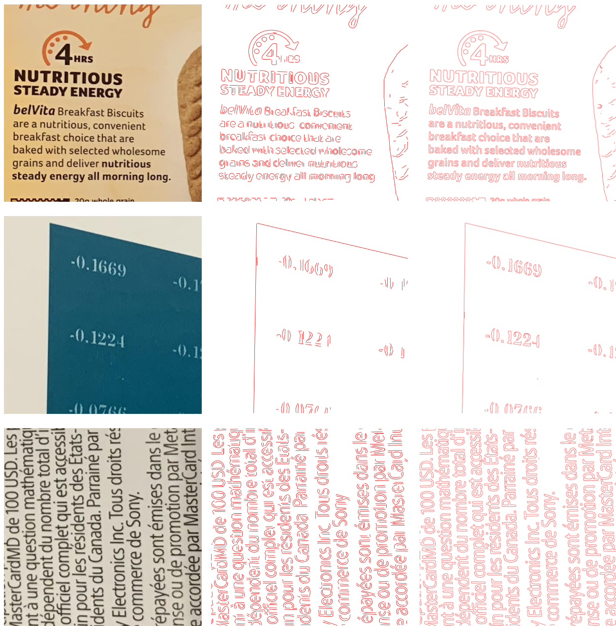
Figure 6.21. Extracting fine curve pixels. From left to right: input image, ELSDc [27] and our curve pixel detection result.
