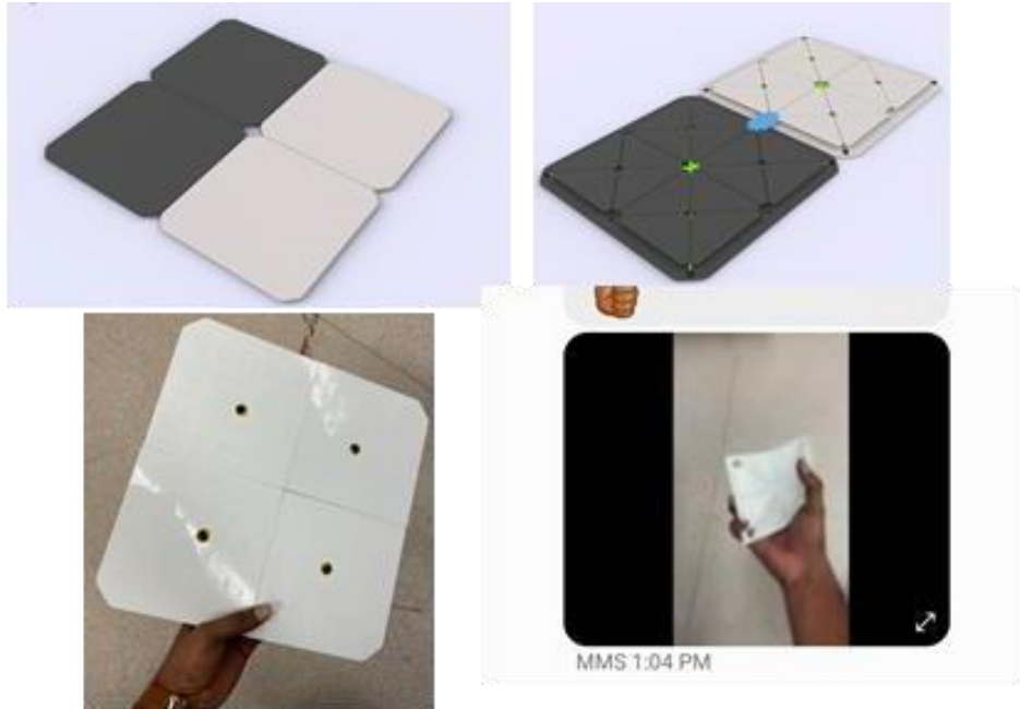
Figure 5.2 Design of a smart pad. Four sensors are radially arranged on a 3D printed plate. 10 mm-wide single fibrous electrodes were used for monitoring human behavior and an object. Each plate can be assembled to form a sensor array.
