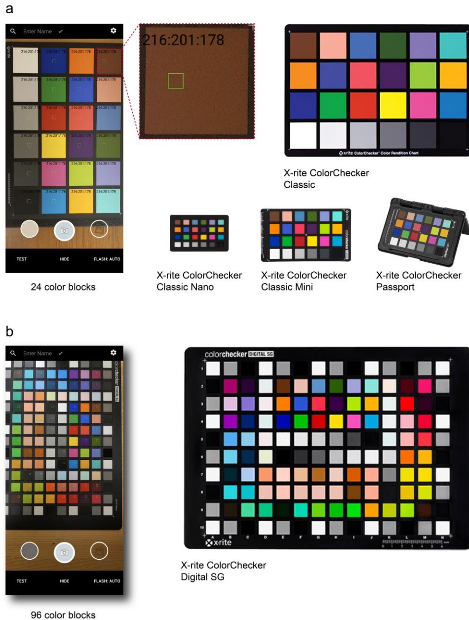
Figure 5. 3. Interfaces of the “24 blocks” and “96 blocks” calibration pages and compatible color charts for these options.
