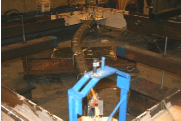
Figure 5.116 Brace In-Plane Buckling - B3
