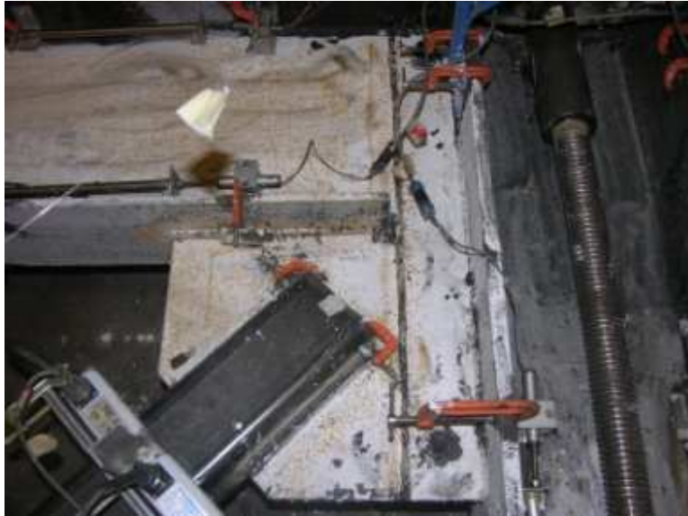
Figure 5.57 North NCBF1-R2 Undamaged Connection
