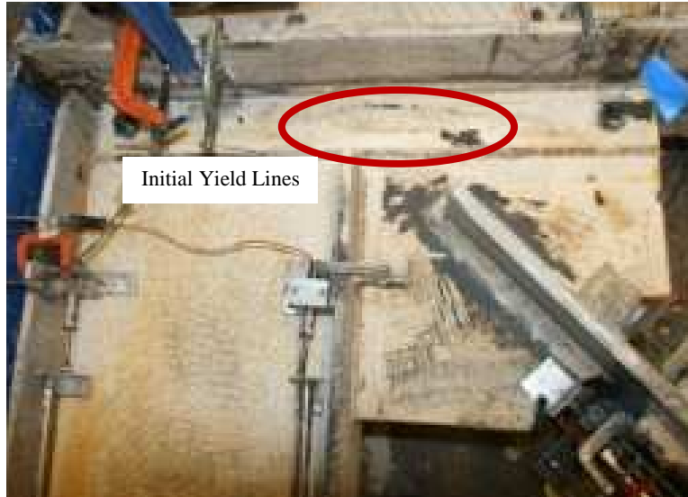
Figure 5.163 South Shear Tab - Y1
