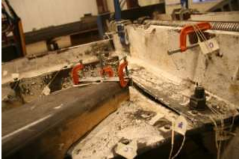
Figure 5.82 Fracture of North Gusset-to-Shear Tab Weld
