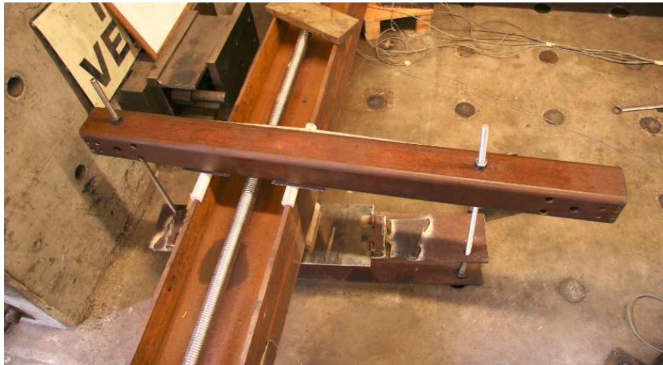
Figure C.6: Out-of-Plane Restraint for East Column
