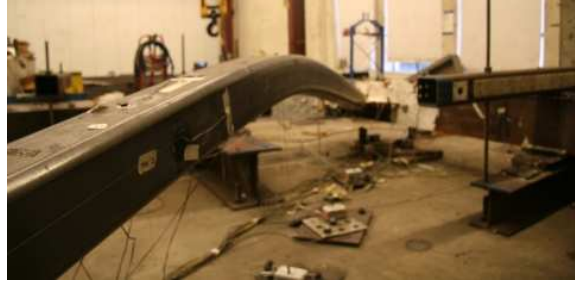
Figure 5.71 Brace Buckling - B3
