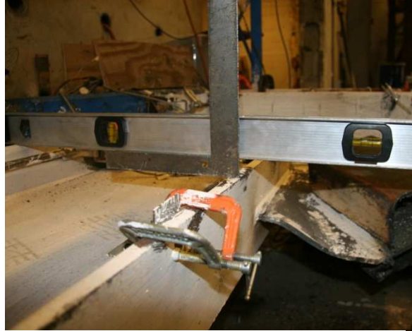
Figure 5.239 Bending of South Beam
