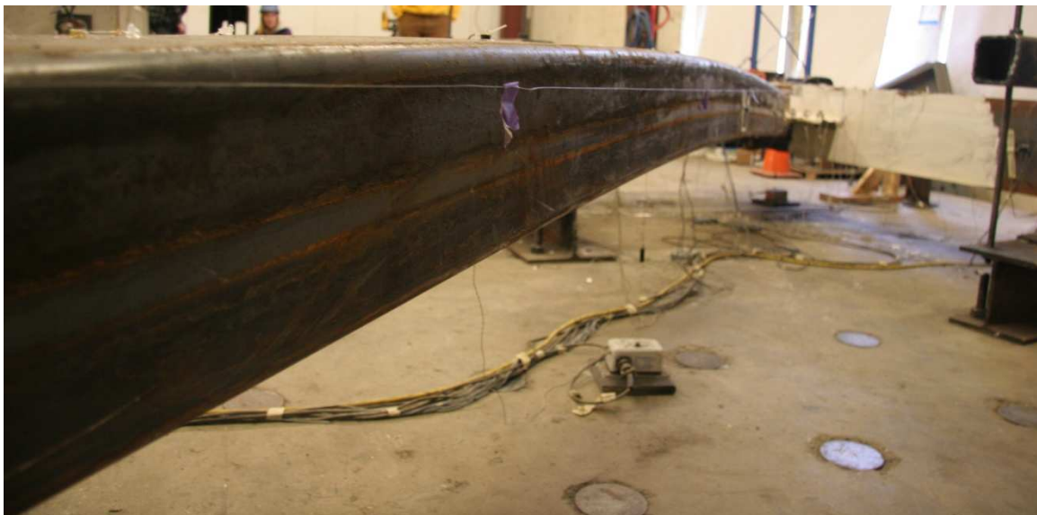
Figure 5.184 Initial Visible Brace Buckling - B1
