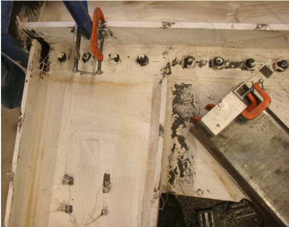
Figure 5.189 Yielding in North Connection
