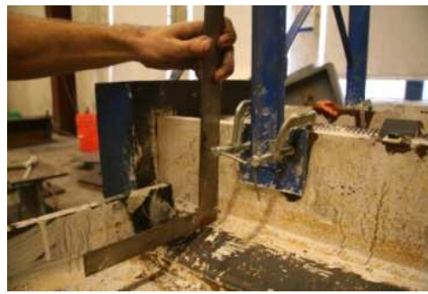
Figure 5.133 Downward Bending of N Shear Tab
