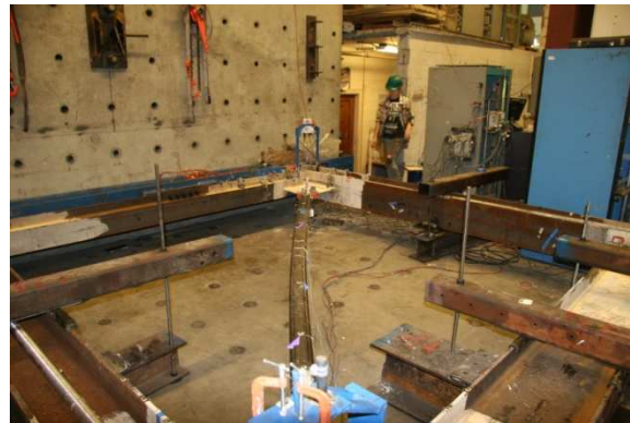
Figure 5.149 In-Plane Buckling of Brace - B1
