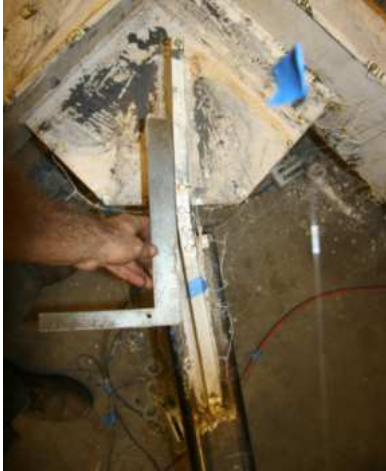
Figure 5.168 North Knife Plate Bending
