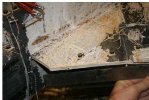
Figure 5.111 Upward Bending of S Gusset Plate
