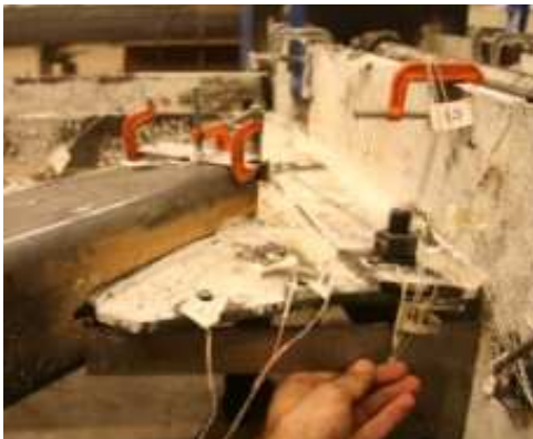
Figure 5.74 Bending of North Gusset Plate
