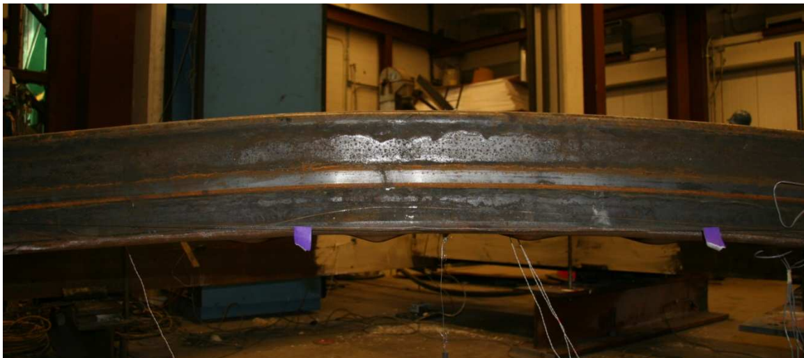
Figure 5.196 Bulging of Brace Bottom Flange
