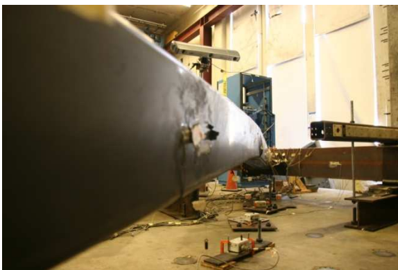
Figure 5.37 Brace Buckled Shape at Cupping
