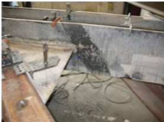
Figure 6.27 Column Flange Yielding (Powell 2010)
