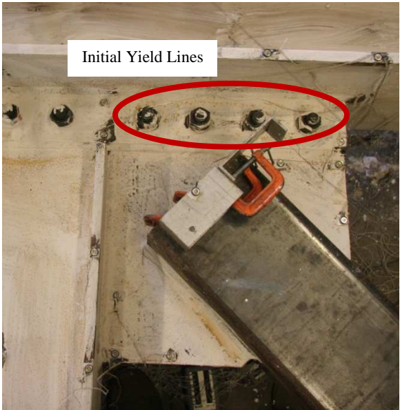
Figure 5.181 Yielding in North Shear Tab
