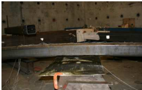
Figure 5.109 Brace Upward Out-of-Plane Buckling
