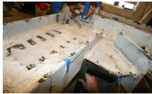
Figure 5.153 Downward Bending of S Gusset Plate Figure 5.154 Downward Bending of N Gusset Plate
