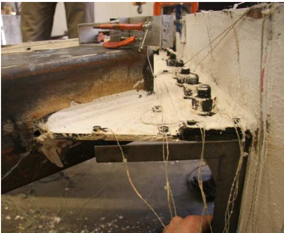
Figure 5.176 Upward Bending of N Gusset
