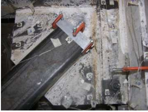
Figure 5.68 North Gusset Plate and North Shear Tab - Y2
