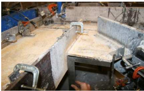
Figure 5.153 Downward Bending of S Gusset Plate Figure 5.154 Downward Bending of N Gusset Plate
