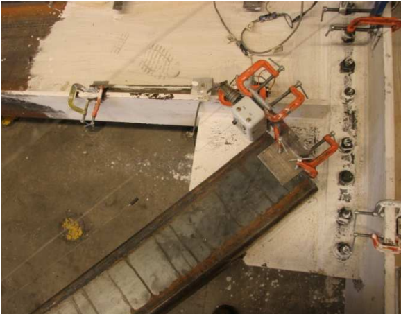
Figure 5.190 Yielding in South Connection
