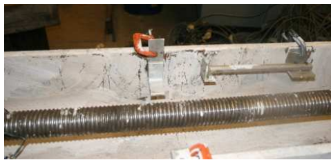
Figure 5.124 Yielding of West Column
