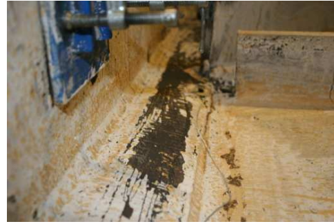
Figure 5.121 Downward Bending of N Shear Tab
