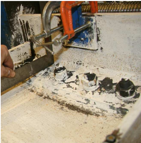
Figure 5.218 Bending of North Shear Tab
