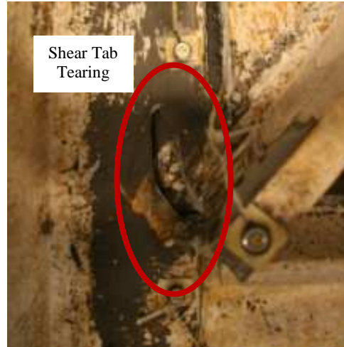
Figure 5.135 Increased MT of North Shear Tab
