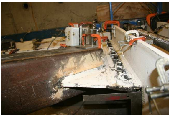
Figure 5.213 Bending of South Gusset Plate
