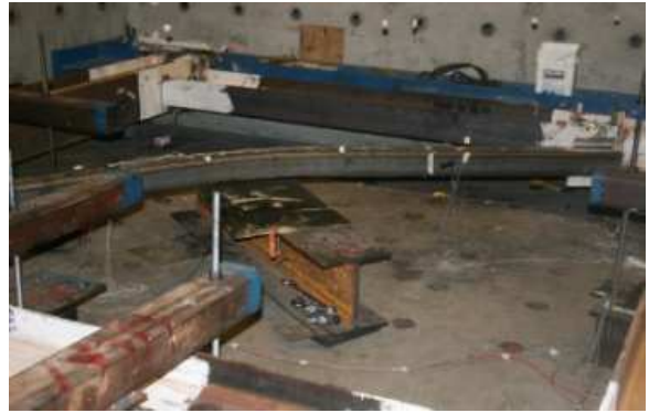
Figure 5.117 Brace Out-of-Plane Buckling - B3
