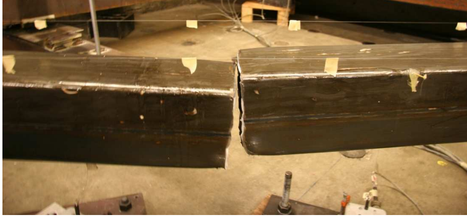
Figure 5.13 Brace Fracture - BF NCBF1
