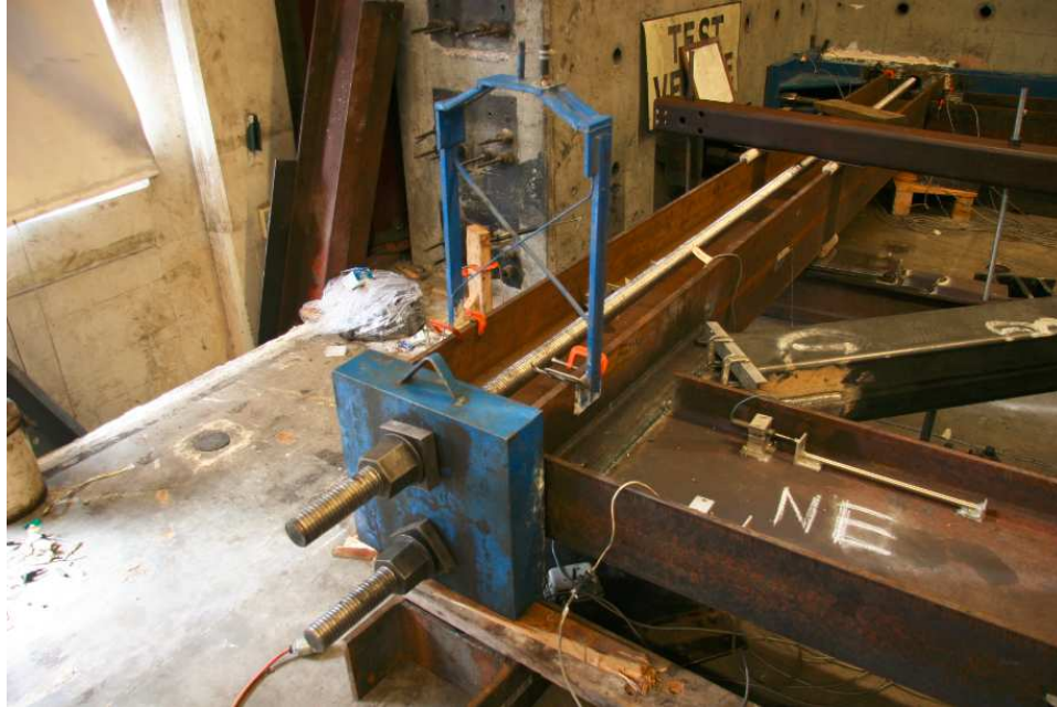
Figure C.4: East Column Cap Plate and Axial Load Rods
