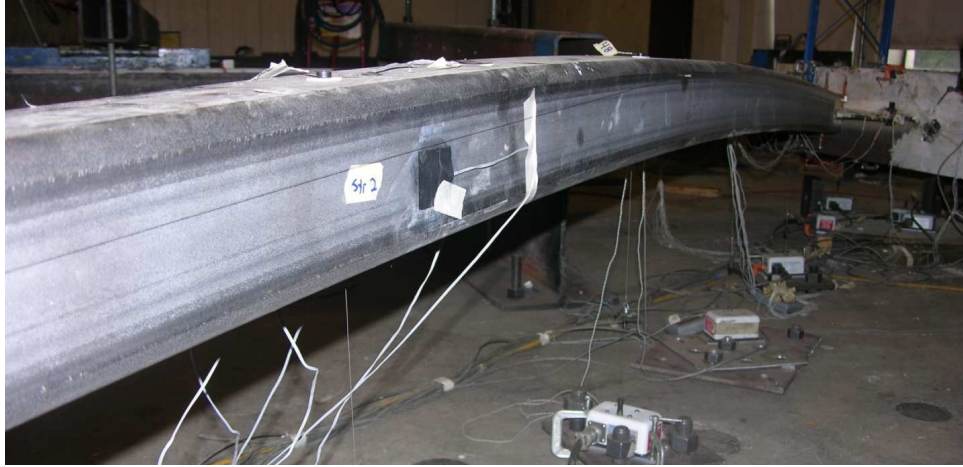
Figure 5.9 Initial Brace Global Buckling - B1 NCBF1-R2
