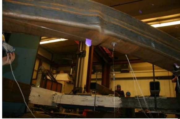
Figure 5.216 Brace Cupping - BC
