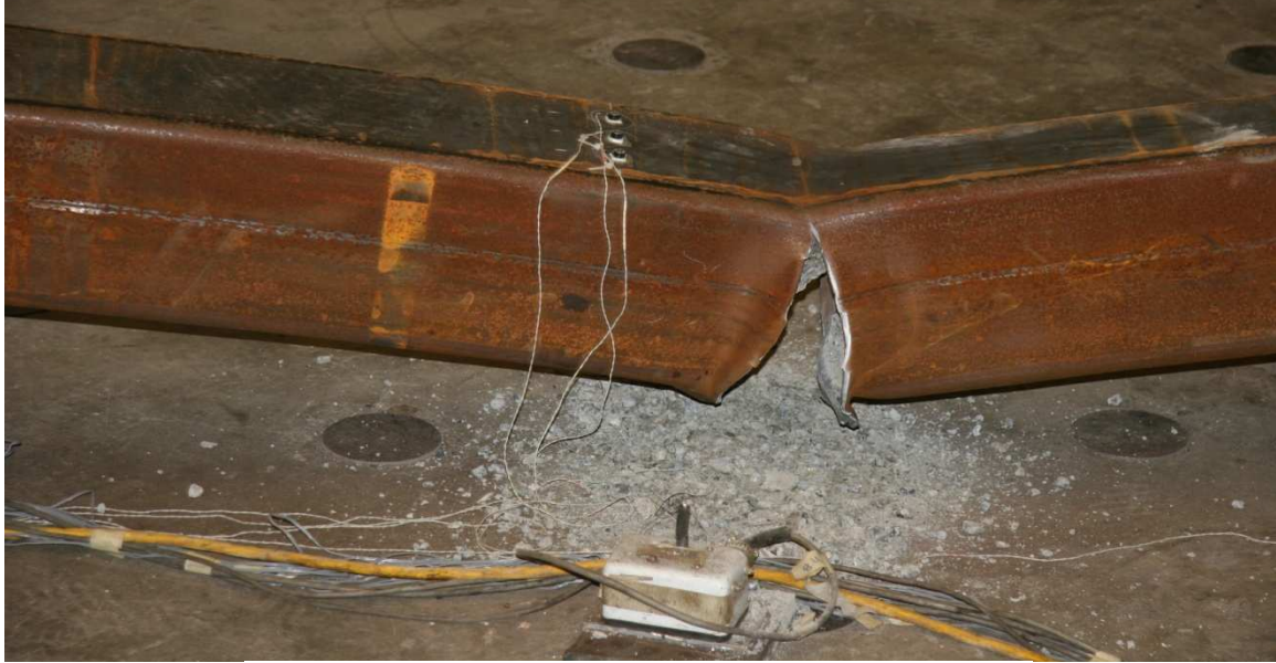
Figure 5.234 Maximum Downward Brace Deflection
