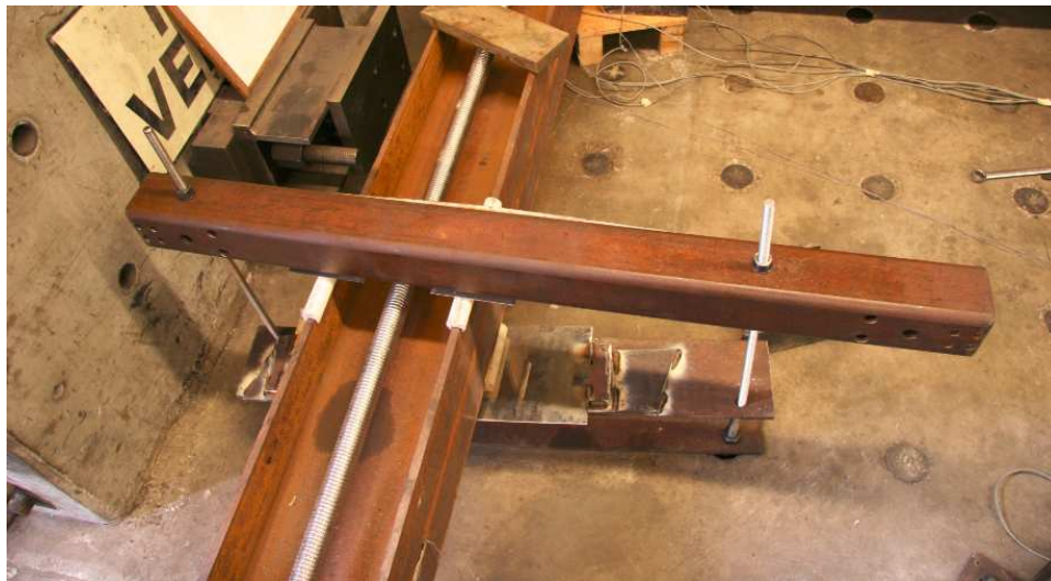
Figure 4.5 East Column Out-of-Plane Restraint
