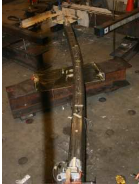
Figure 5.98 Brace In-Plane Buckling - B1
