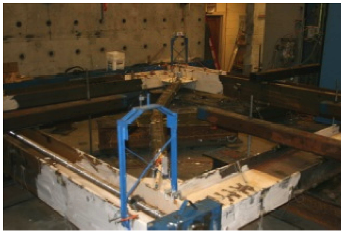
Figure 5.104 Brace Buckling - B2
