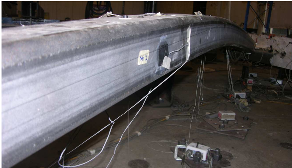
Figure 5.10 Moderate Brace Global Buckling - B2 NCBF1-R2
