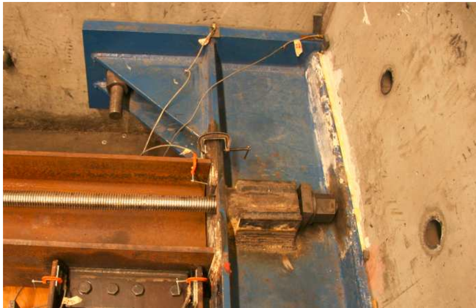
Figure C.5: Axial Load Rod Anchor for East Column
