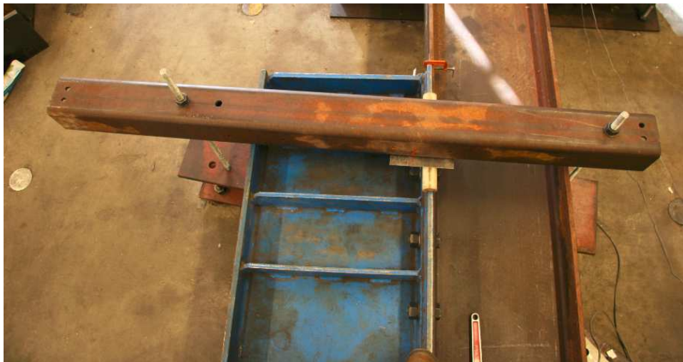
Figure C.8: Out-of-Plane Restraint Load Beam
