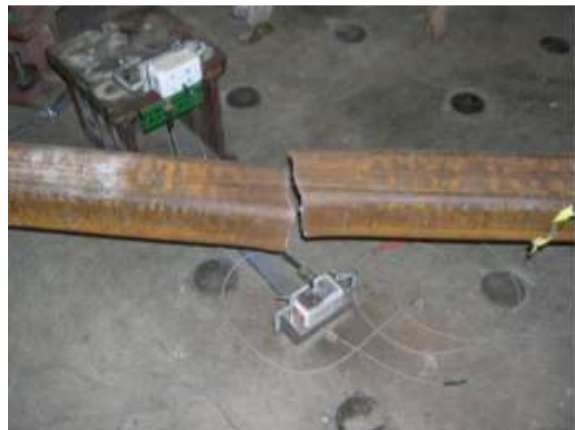
Figure 2.7 HSS18 Brace Fracture (Powell 2010)
