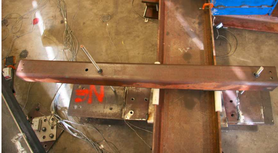
Figure C.9: Out-of-Plane Restraint for North Beam
