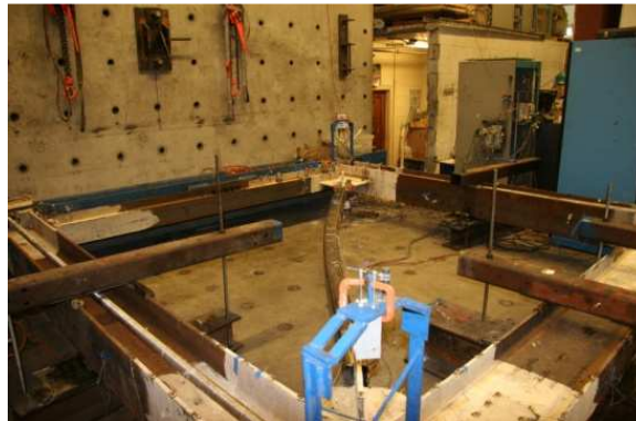
Figure 5.156 Brace In-Plane Buckling - B2
