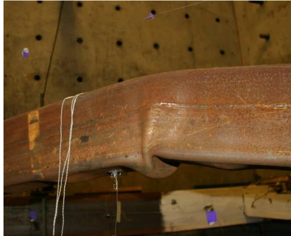
Figure 5.221 Increased Brace Cupping
