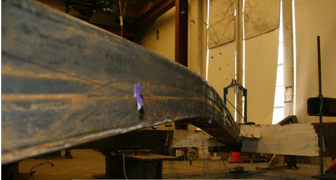
Figure 5.198 Moderate Brace Buckling - B2
