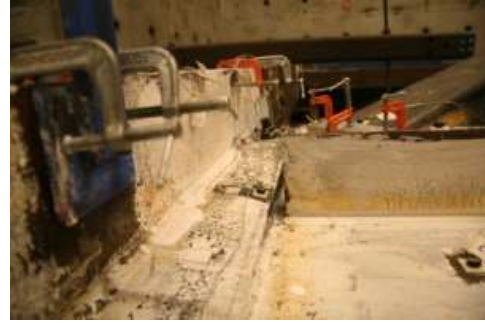
Figure 5.83 Downward Bending of N Shear Tab
