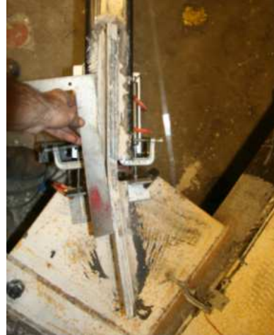
Figure 5.169 South Knife Plate Bending
