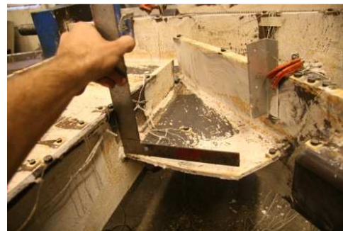
Figure 5.126 Downward Bending of N Shear Tab
