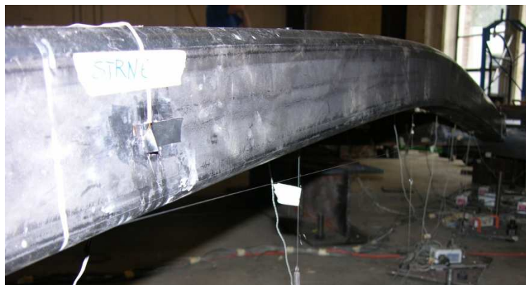
Figure 5.51 Brace Buckling - B2
