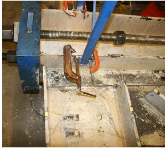
Figure 5.171 North Beam Flange Bearing on North Shear Tab
