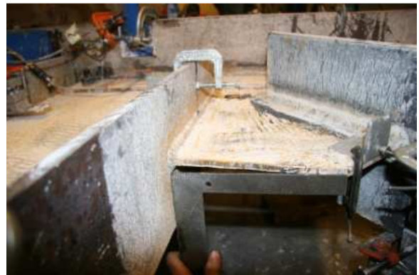
Figure 5.162 South Gusset Plate Bending
