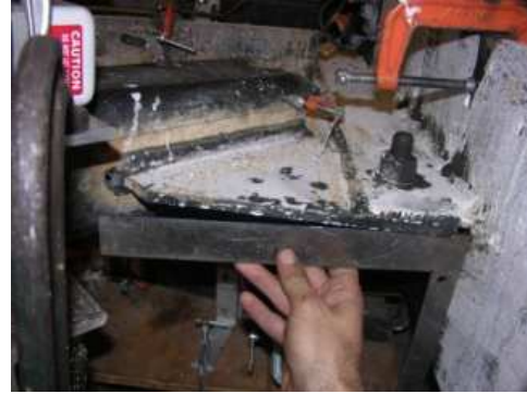
Figure 5.63 South Gusset Plate Bending
