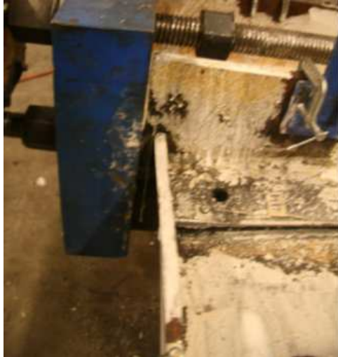
Figure 5.85 North Beam Bearing on North Shear Tab
