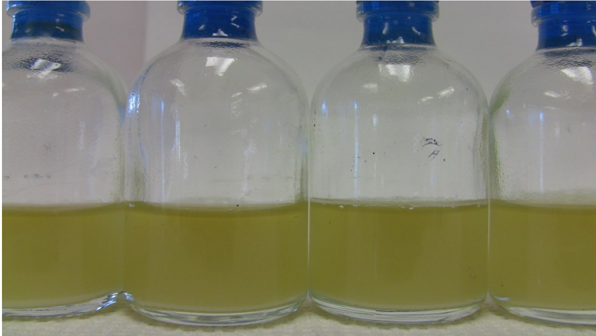
Figure 4 Group A. 50 mL serum bottles filled with 20 mL slurry.
