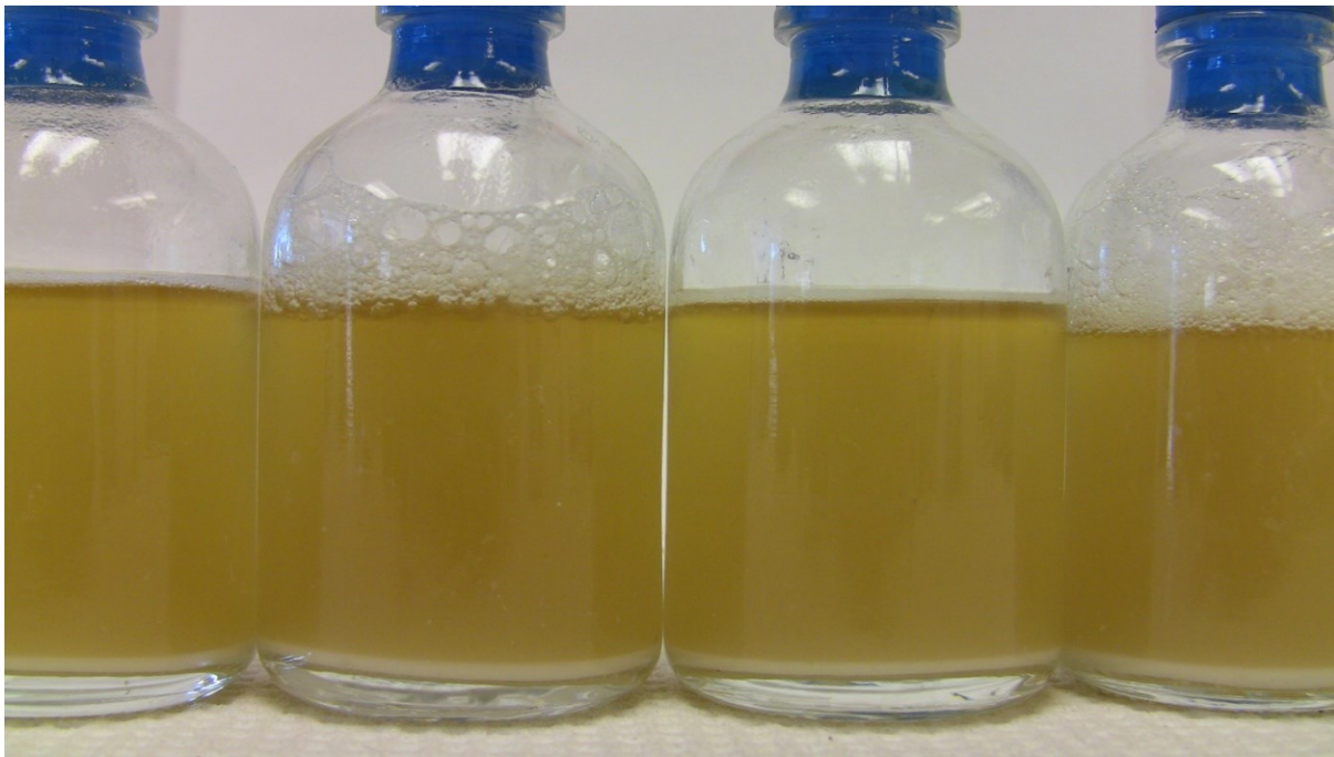
Figure 4 Group A. 50 mL serum bottles filled with 20 mL slurry.
