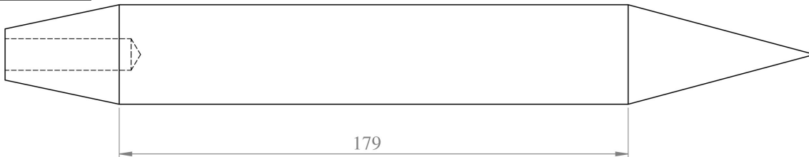
Figure 3.3: A P380 projectile with 1.7, 3, and 5 baffle length shoulders. The nose and tail-cone geometry is identical for each.
