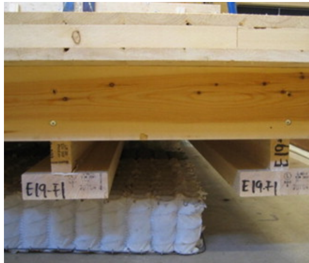
Figure 2.7: CLT Laboratory Setup [ Jarnerö et al., 2015 ]
