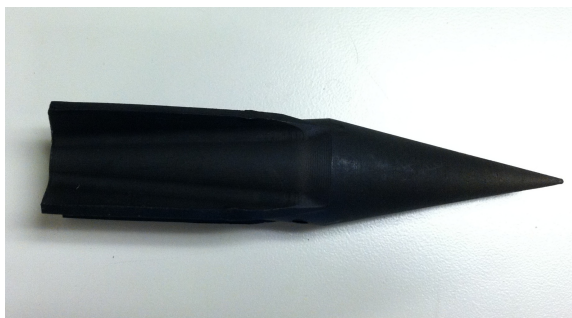
Figure 5.3: Type D polycarbonate projectile caught with gas dynamic catcher
