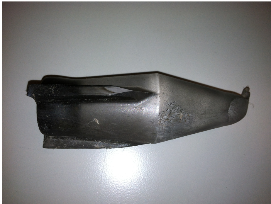
Figure 4.7: Type A polycarbonate projectile after an unsuccessful shot with “bulge” on back end
