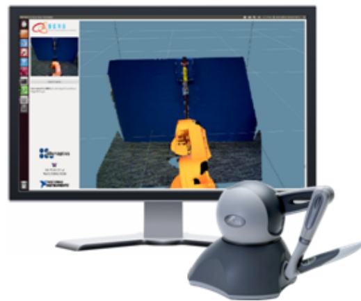
Figure 5.2: Teleoperation master console station. Includes 3DOF haptic device as well as a LCD monitor to display visual feedback.
