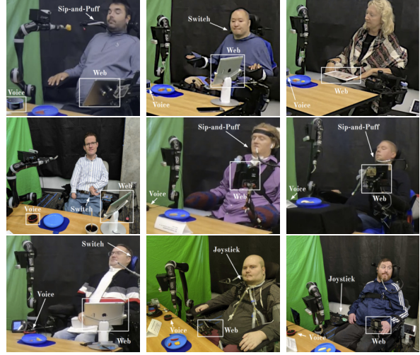
Figure 2.1: Participants with mobility impairments with options for the voice interface using Alexa and web-interface displayed in their/our tablets mounted in different positions according to their preference or constraints of system integration. When needed a switch was installed to control the web interface.
