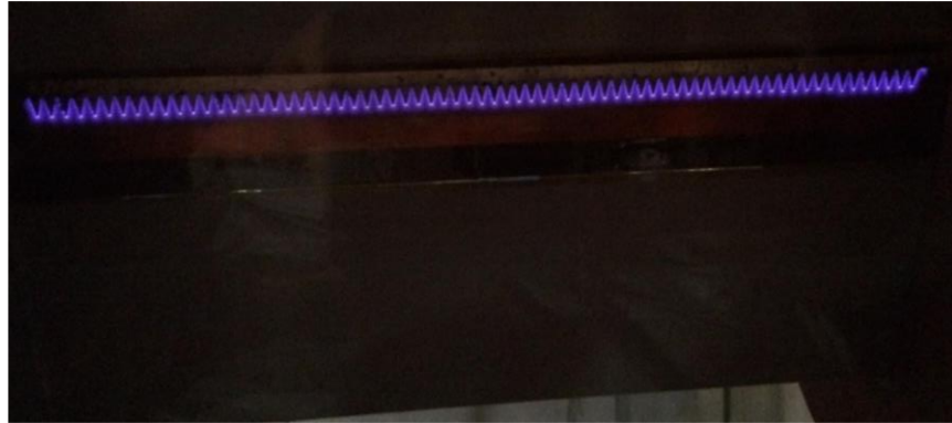
Figure A.4. DBD operating on an airfoil.
