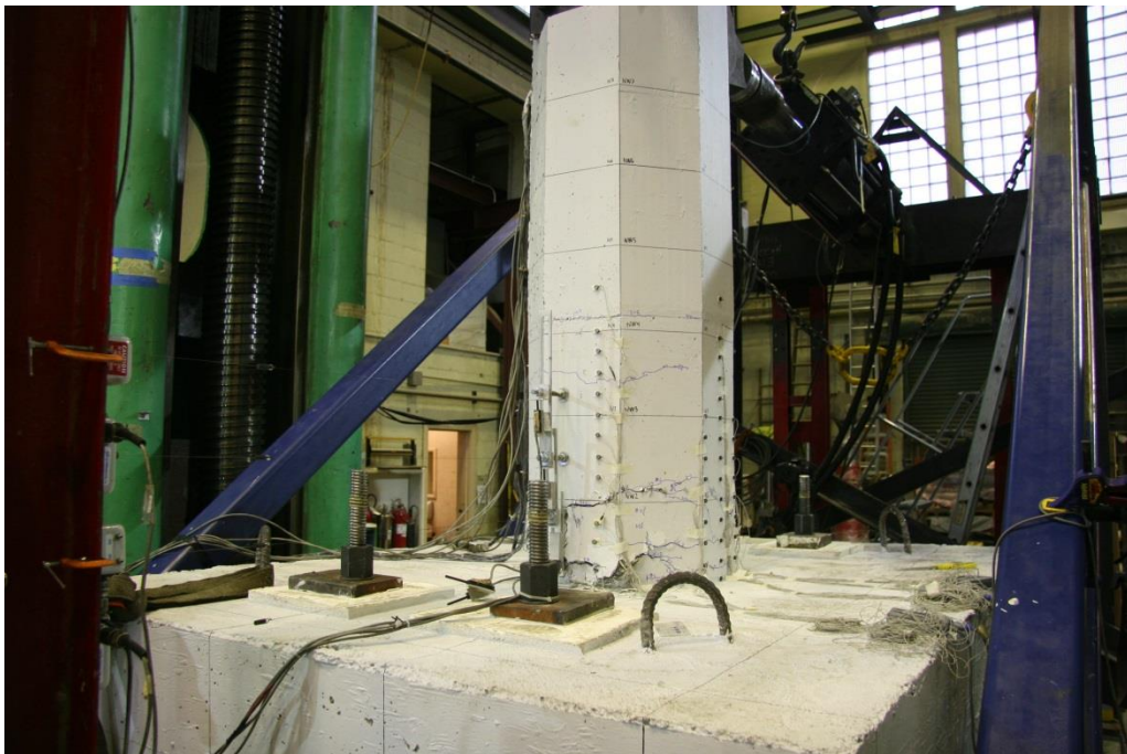
Figure C - 3: Column fully spalled, cycle 9-1.
