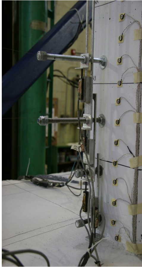
Figure 3-6: Curvature rod tracking system.
