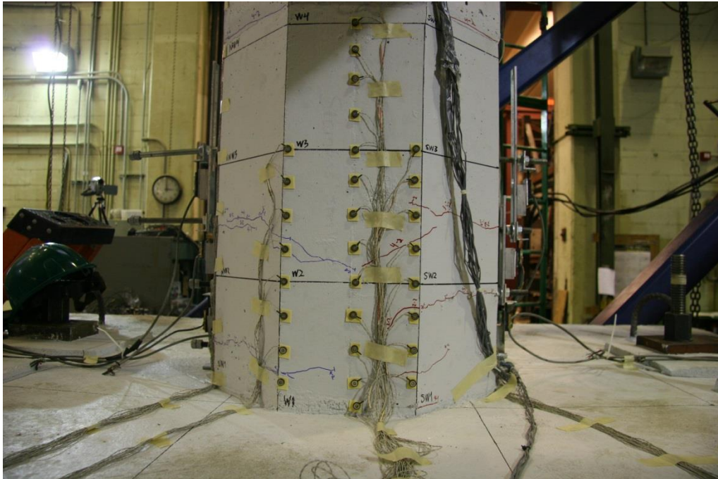
Figure C - 9: First open residual crack, cycle 5-2.
