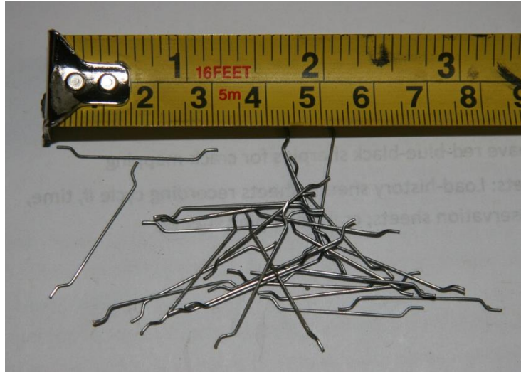
Figure 2-6: Dramix ZP 305 steel fibers.
