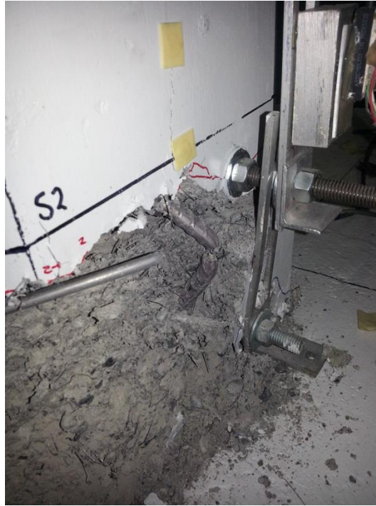
Figure 4-10: PreT-SS broken longitudinal rebar and broken spiral after spalled concrete had been peeled off after the test was finished.
