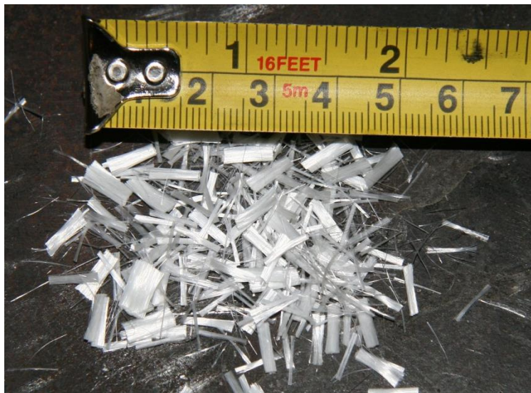
Figure 2-7: Kuralon RECS 15x8mm polymer fibers.
