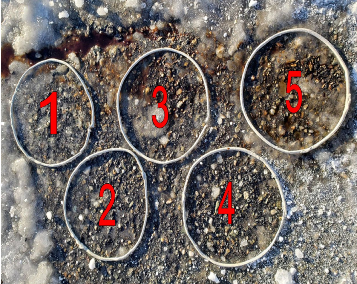
Figure 3.2 Example test site with rope caulk barriers
