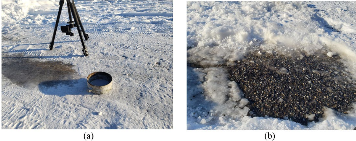
Figure 2.2 Testing conditions with (a) hardpack present and (b) hardpack removed to simulate a well-maintained road.
